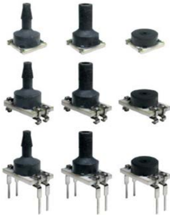
Figure 7: The Honeywell NBP Series Board Mount Pressure Sensors are uncompensated, unamplified sensors that measure absolute and gauge pressures. They are intended for use with noncorrosive, non-ionic gases.
