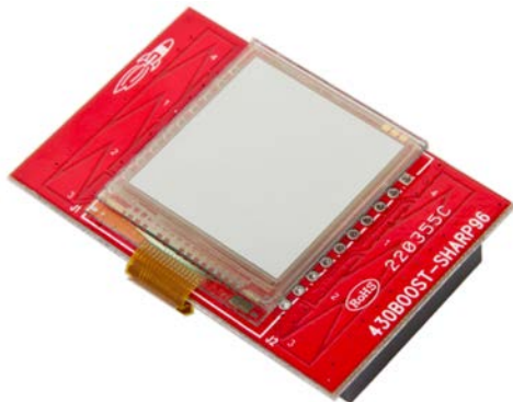
Figure 8: The 430BOOST-SHARP96 Sharp LCD BoosterPack is the display used for the Tricorder. It is 1.35-inch display offering 96 x 96 pixels that can be controlled over the SPI bus.
