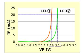
Therefore, 1 resistor per LED can reduce difference of current value to have uniform luminous intensity.
