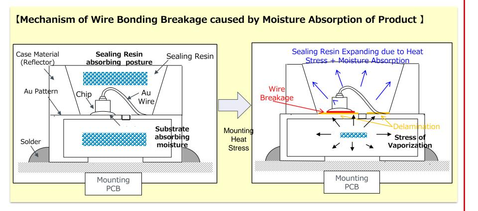
When the product is absorbing the moisture, the vaporized stream (by the heat of reflow)will go out, its stress will lift up the sealing resin from the bottom and result in breakage of wire bonding.
