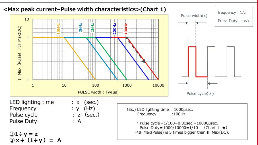
IF Max(in case of Pulse duty10%) is 5 times bigger than IF Max(DC).
