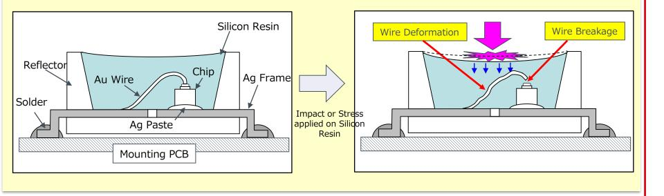
When it is mounting, please have the adsorption collet touching with reflector. After it is mounted, please be care to handle with the part of sealing.
