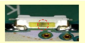
The Ag of frame is corroded and its color changed into black →Low luminous intensity due to low light absorption
