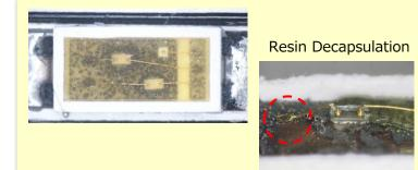
The Ag pattern in the LED case is corroded and color changed into black→wire delamination
