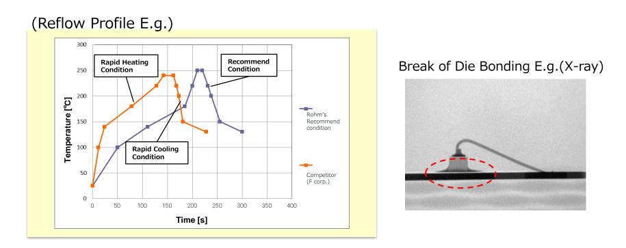
If the peak temperature is too high (excessive), it may cause delamination between Ag paste and circuit board due to warpage of printed wiring circuit board or expansion of resin. And if the temperature gradient of temperature rising/falling is large, it can also cause delamination, so please use it in  $1 \sim 3^{\circ}$ /sec.
