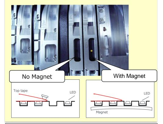
For super small products, it may paste on tape due to static electricity because of the operational environment. In the case, it can solve the problem by installing a magnet on the mounting machine.
