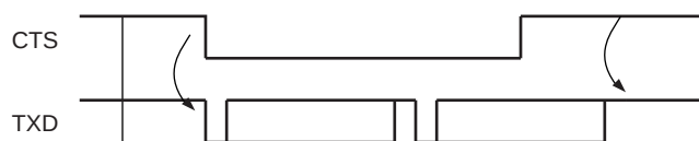
Figure 43-28. Transmitter Behavior when Operating with Hardware Handshaking
