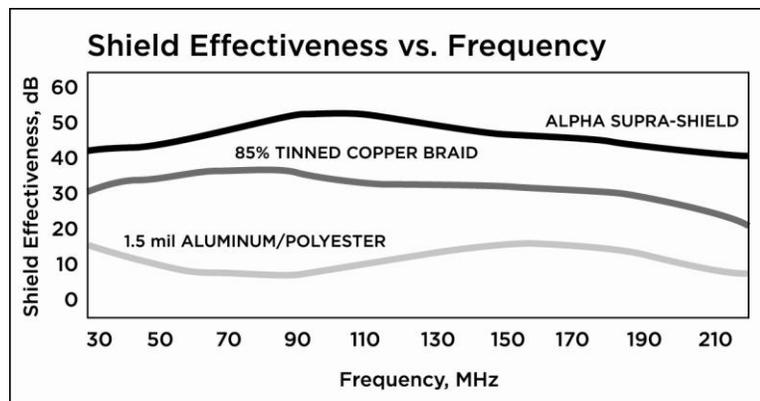
**Figure 3. Foil-braid shielding yields the best shielding effectiveness**
