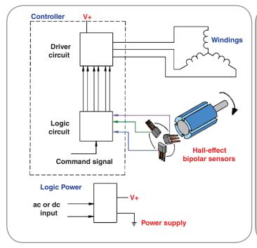
Bipolar Hall-effect sensors are used in BLDC motors to detect the position of the rotating magnet. In this example, an eight-pole motor with a three-phase winding uses three bipolar latching Hall-effect sensors.
