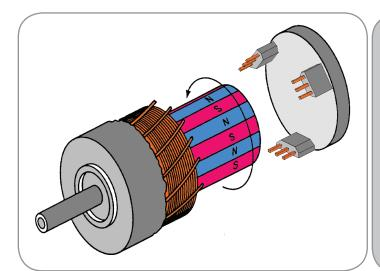
BLDCs use electronic commutation to control the power distribution to the motor, using Hall-effect sensors to measure the motor's position.
