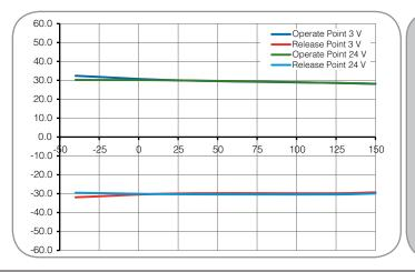
The Honeywell SS360ST, SS360NT, and SS460S bipolar latching Hall-effect sensors offer reliable switching points over its operating temperature range of -40 °C to 150 °C.
