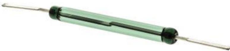
In a normally open (NO) application the contacts are normally separated, and when you bring a magnet up to the switch the 2 contacts become opposite magnetic poles, which causes the leads to attract and snap together.
