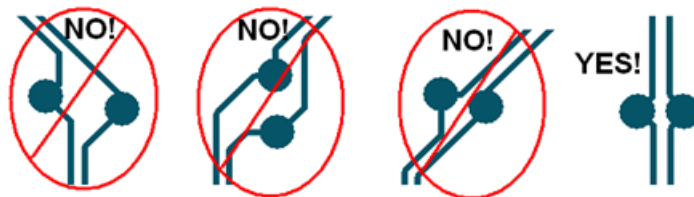
Figure 16 • Example of Asymmetric and Symmetric Differential Pairs Structure
