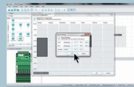
3.12. To carry out a simulation, select a suitable time interval.
