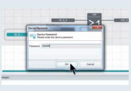
5.2. Once a connection has been established to the logic module, a password is requested. Enter the password set in step 2.4. here.
