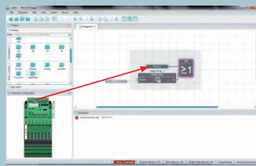
3.7. Insert input DI\_0\_0 by means of drag & drop and connect it to the OR block. Connect input DI\_0\_1 to the week timer.
