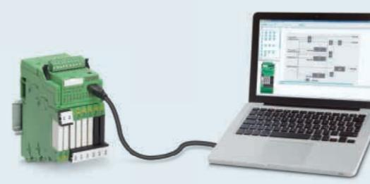
1.3. Following successful installation, connect the logic module to your computer via a USB cable and supply it with a voltage of 24 V. The hardware driver is installed automatically. If you do not want to connect the hardware yet, please proceed directly with program creation (3).
