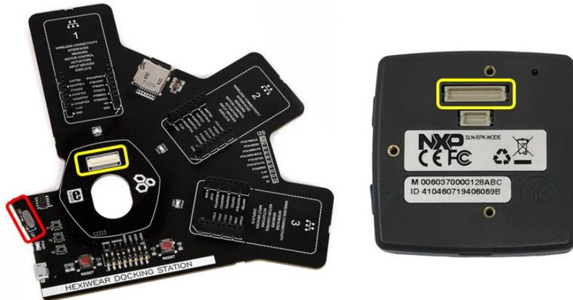
Figure 66. Docking station connector
