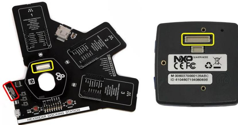
Figure 108. Docking station connector
