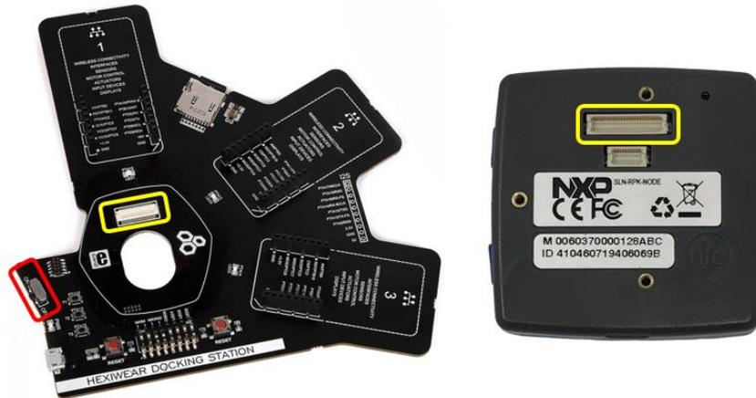
**Figure 108. Docking station connector**
