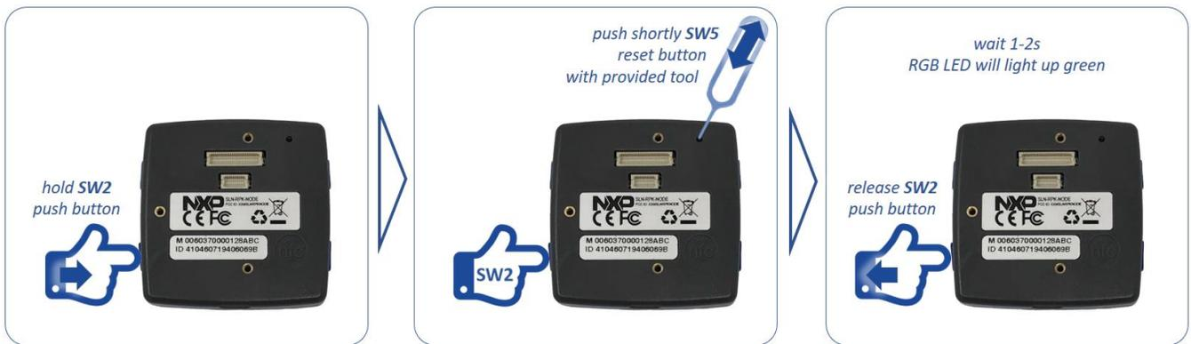
Figure 163. Instructions for KW41Z application recovery
