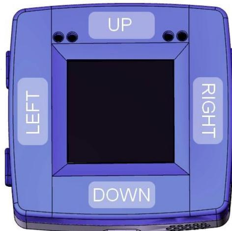
Figure 100. Touch electrodes location
