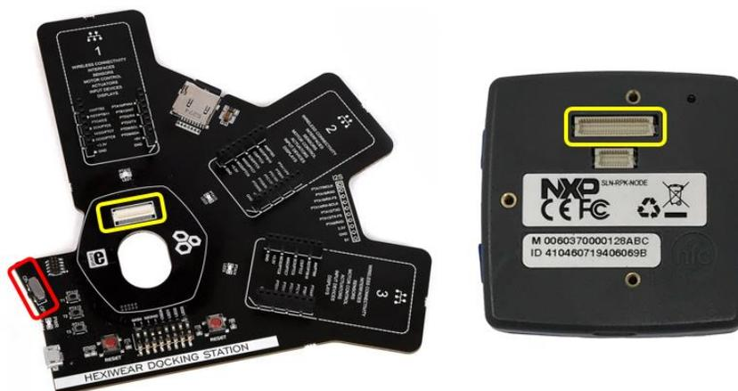
**Figure 182. Docking station connector**
