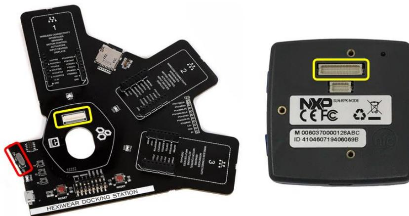
Figure 171. Docking station connector
