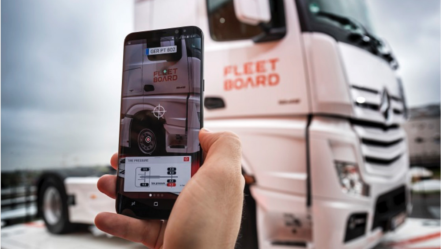
Figure 4: FleetBoard Vehicle Lens app is a pilot project that tracks a truck’s number plate and superimposes the information in augmented reality. (Source: FleetBoard)
