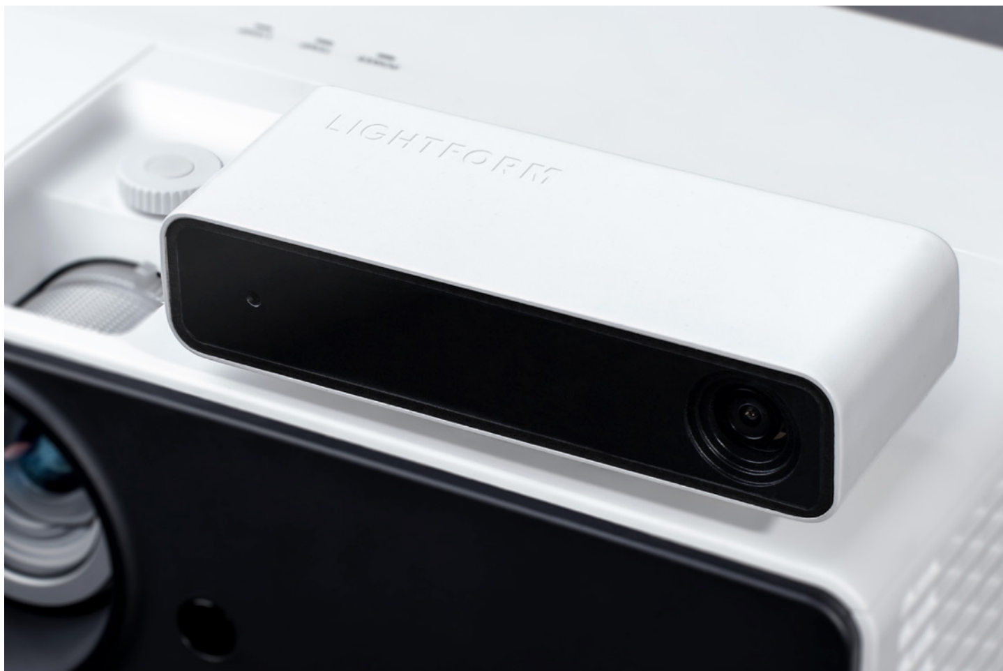
Figure 3: This device connects to any projector to create augmented reality elements for retail, home or office use. (Source: Lightform)
