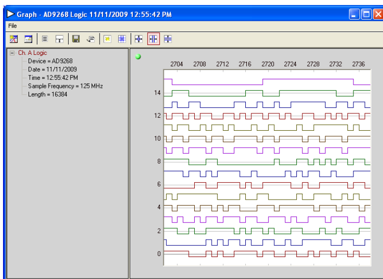
Figure 11. AD9268 ADC with Bit 9 and Bit 10 Shorted Together
