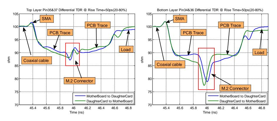
Impedance results met requirement of 850hm connection system.
