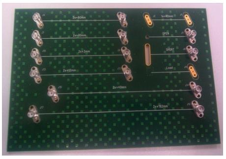
M.2 PCIe connector SI test fixture
