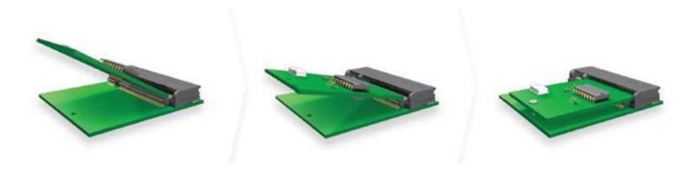
Step 1: Move the module against the housing's chamber
