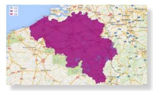
LoRaWAN<sup>™</sup> have a link budget greater than any other standardized communication technology. The link budget, typically given in decibels (dB), is the primary factor in determining the range in a given environment. Above is the coverage map from the Proximus network deployed in Belgium. With a minimal amount of infrastructure, entire countries can easily be covered.
