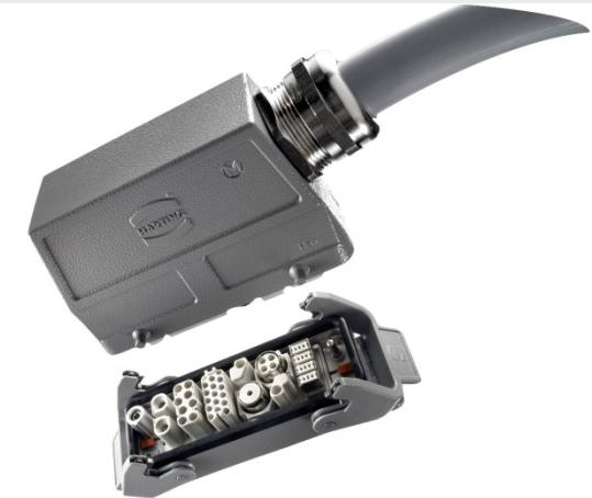
Rectangular connectors have smaller minimum spacing requirements. A circular connector requires sufficient space for a hand to grip it when mating and un-mating. Rectangular connectors can be gripped by the ends or sides. Locking levers can be located on either the ends or side(s). Many large users set their own minimum requirements, based on experience, that invariably require wider spacing for circular connectors.
