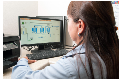
Figure 1: A SCADA network allows an operator to monitor the status of arsenic removal system absorber vessels in a water treatment plant.
