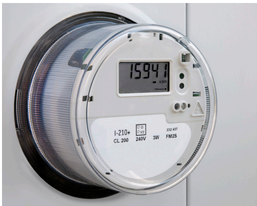
Figure 1: There are already nearly 70 million “smart” electricity meters in the U.S., each one transmitting periodic usage updates typically via a LPWAN but soon via cellular networks as well.
