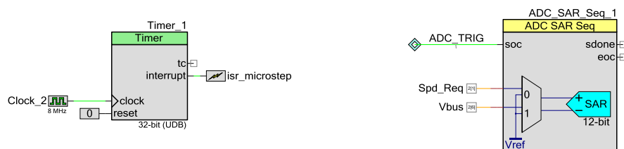
Figure 5-57. ADC,Button and Microstep Timer Schematic
