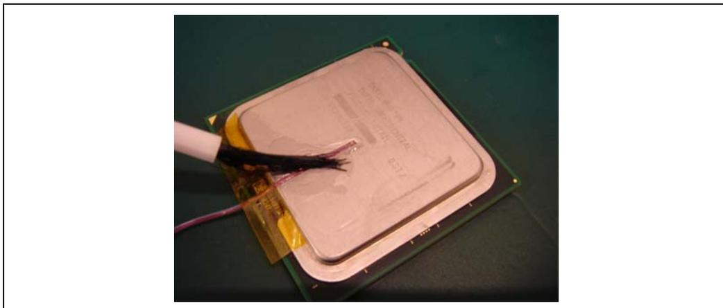
Figure 53. Removing Excess Adhesive from IHS
