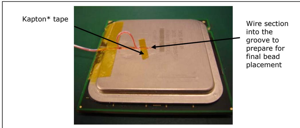
Figure 39. Detailed Thermocouple Bead Placement
