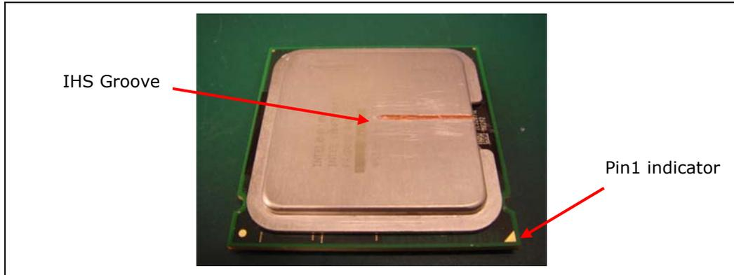
When the processor is installed in the LGA775 socket, the groove is parallel to the socket load lever, and is toward the IHS notch, as shown in Figure 33.
