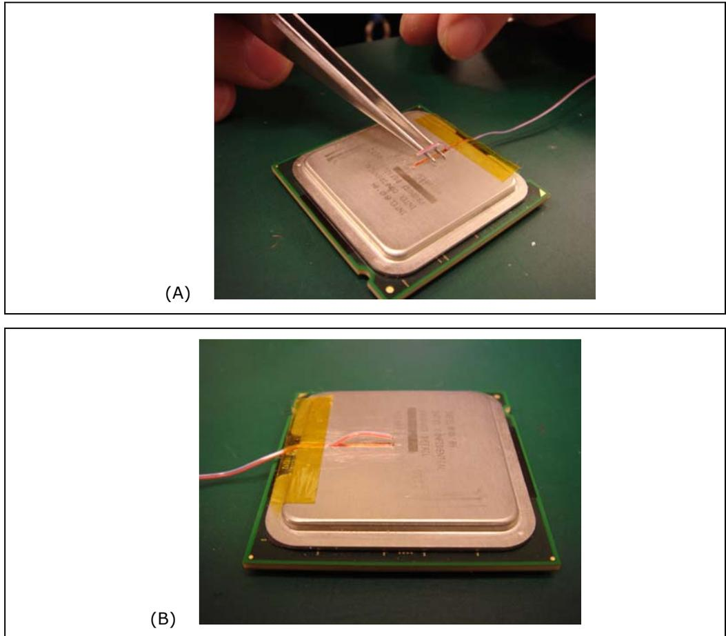
10. Place the package under the microscope to continue with process. It is also recommended to use a fixture (like processor tray or a plate) to help holding the unit in place for the rest of the attach process.
