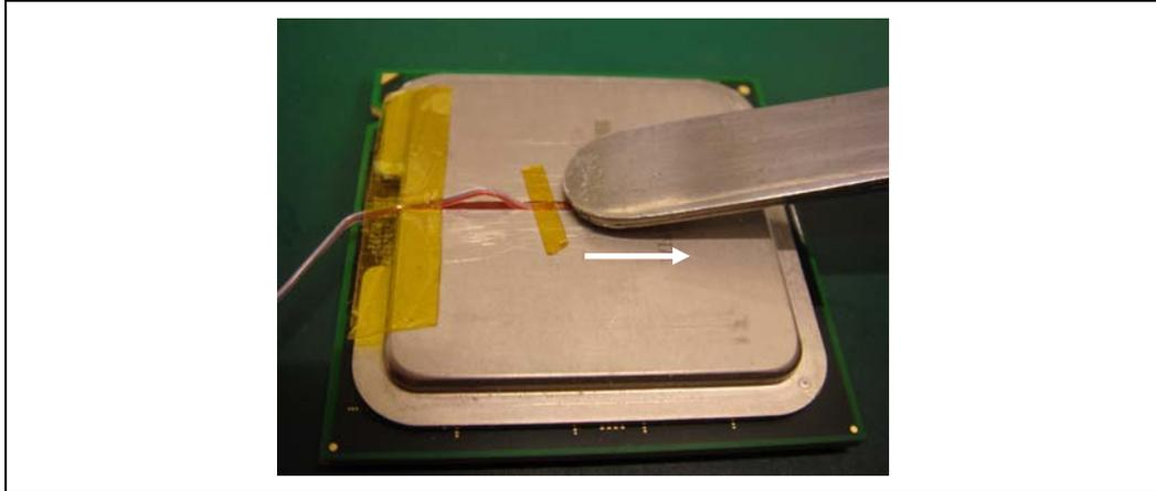
26. Allow the device to cool down. Blowing compressed air on the device can accelerate the cooling time. Monitor the device IHS temperature with a handheld meter until it drops below 50° C before moving it to the microscope for the final steps.
