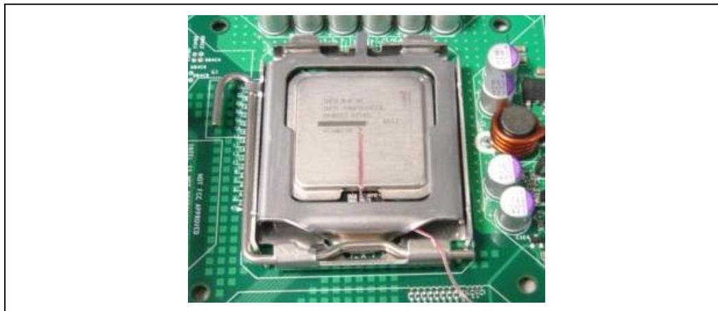
Select a machine shop that is capable of holding drawing specified tolerances. IHS groove geometry is critical for repeatable placement of the thermocouple bead, ensuring precise thermal measurements. The specified dimensions minimize the impact of the groove on the IHS under the socket load. A larger groove may cause the IHS to warp under the socket load such that it does not represent the performance of an ungrooved IHS on production packages.
