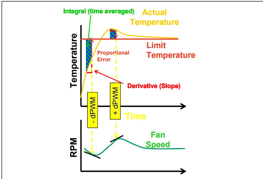
For a PID algorithm to work, limit temperatures are assigned for each temperature sensor. For Intel QST, the  $T_{\text{CONTROL}}$  for the processor and chipset are to be used as the limit temperature. The ME will measure the error, slope and rate of change using the equations below:
