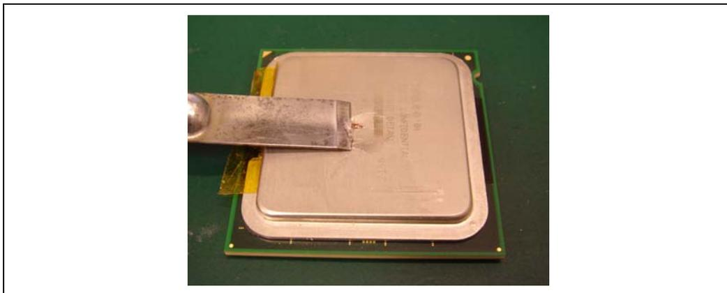
33. Using a blade, carefully shave any adhesive that is above the IHS surface (see Figure 53). The preferred method is to shave from the edge to the center of the IHS.
