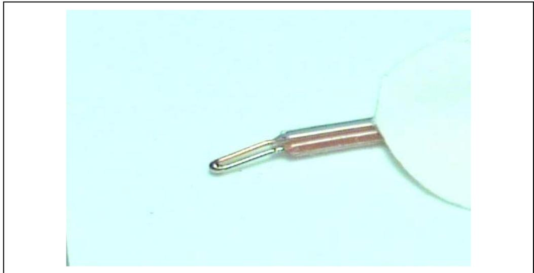
3. Measure the thermocouple resistance by holding both contacts on the connector on one probe and the tip of thermocouple to the other probe of the DMM (measurement should be about ~3.0 ohms for 36-gauge type T thermocouple).
