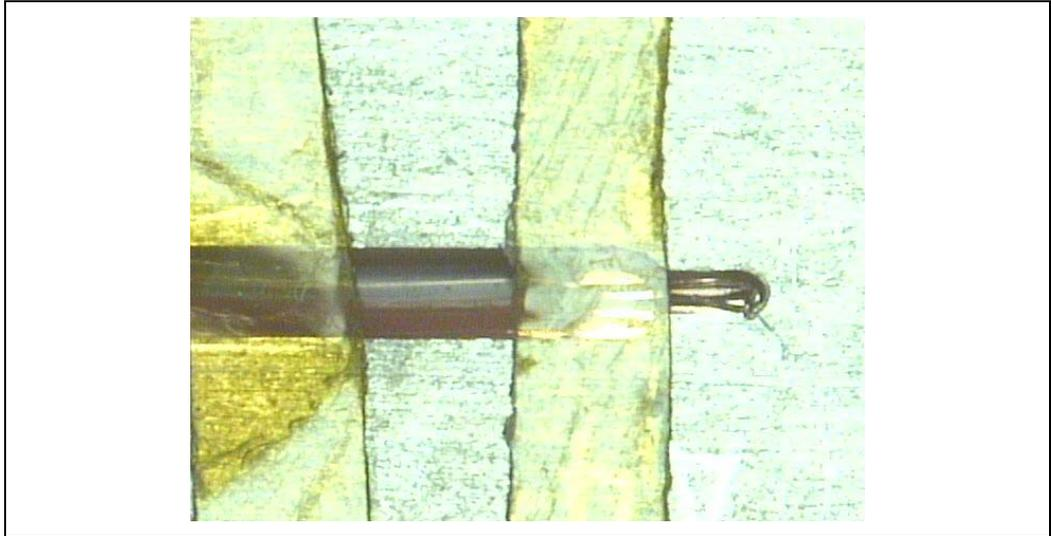
12. Place a 3<sup>rd</sup> piece of tape at the end of the step in the groove as shown in Figure 40. This tape will create a solder dam to prevent solder from flowing into the larger IHS groove section during the melting process.
