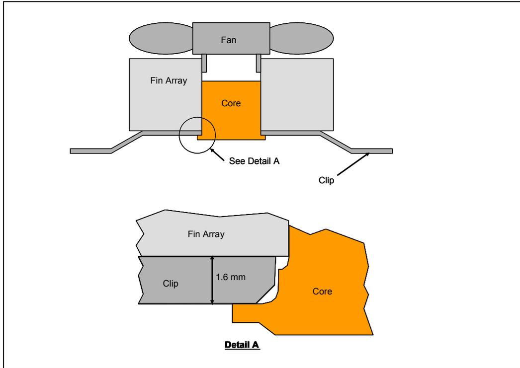
Figure 18. Critical Core Dimension
