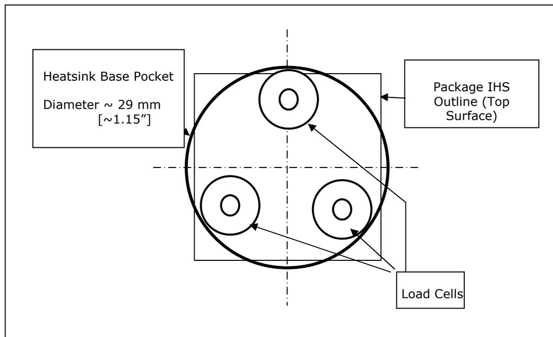
Figure 27. Load Cell Installation in Machined Heatsink Base Pocket (Side View)
