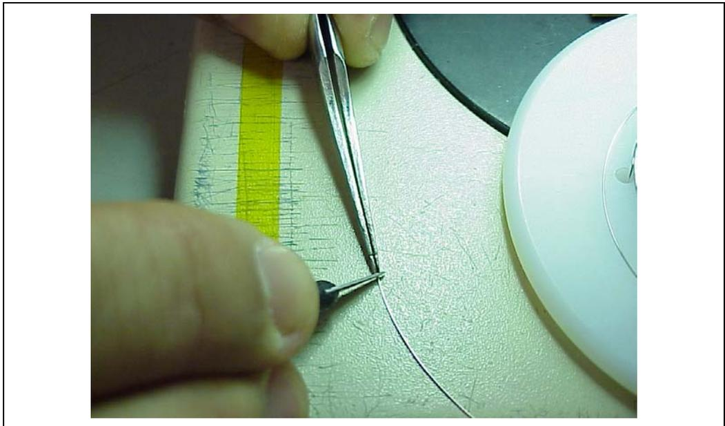
16. Place the two pieces of solder in parallel, directly over the thermocouple bead (see Figure 44)
