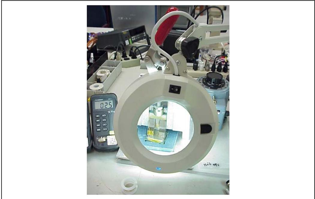
Figure 47. Moving Solder back onto Thermocouple Bead
