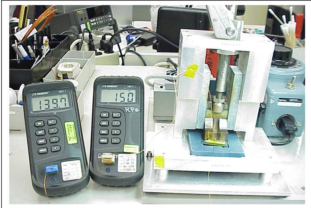
21. Remove the land side protective cover and place the device to be soldered in the solder station. Make sure the thermocouple wire for the device being soldered is exiting the heater toward you.
