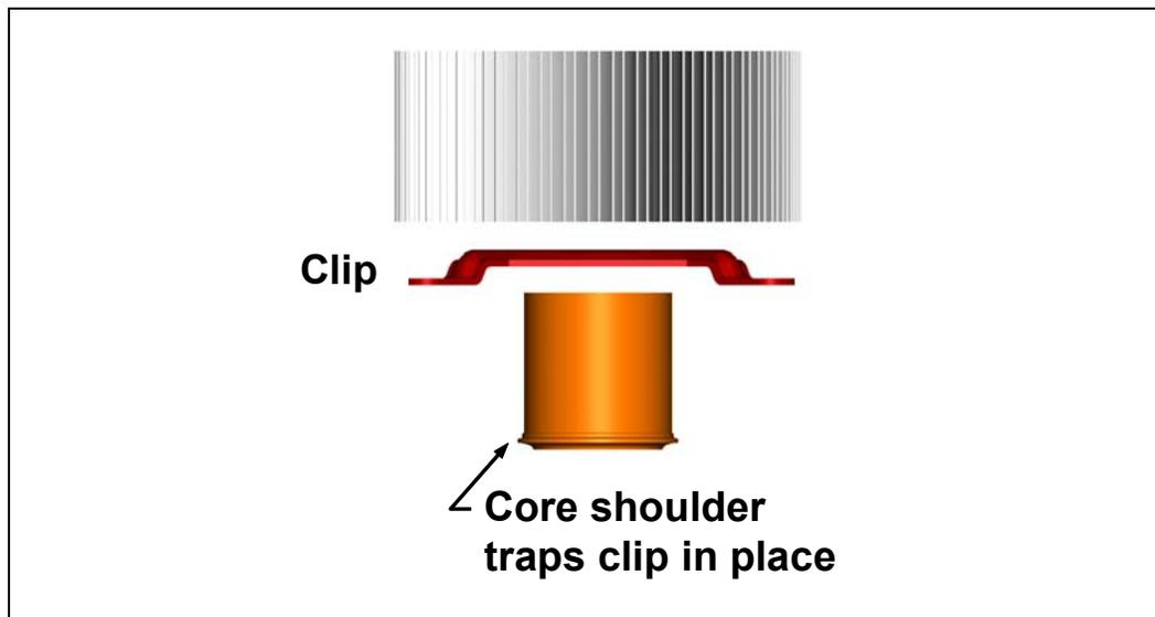
The mechanical interface with the reference attach mechanism is defined in Figure 17 and Figure 18. Complying with the mechanical interface parameters is critical to generating a heatsink preload compliant with the minimum preload requirement provided in Section 2.1.2.2.
