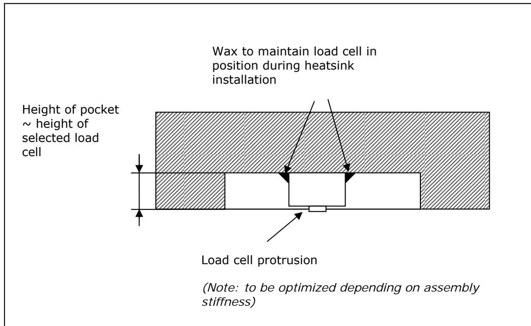
Figure 28. Preload Test Configuration
