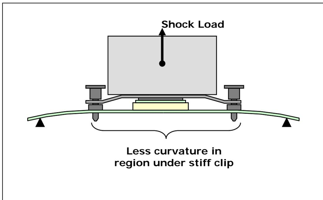
The target metal clip nominal stiffness is 540 N/mm [3100 lb/in]. The combined target for reference clip and fasteners nominal stiffness is 380 N/mm [2180 lb/in]. The nominal preload provided by the reference design is 191.3 N ± 44.5 N [43 lb ± 10 lb].
