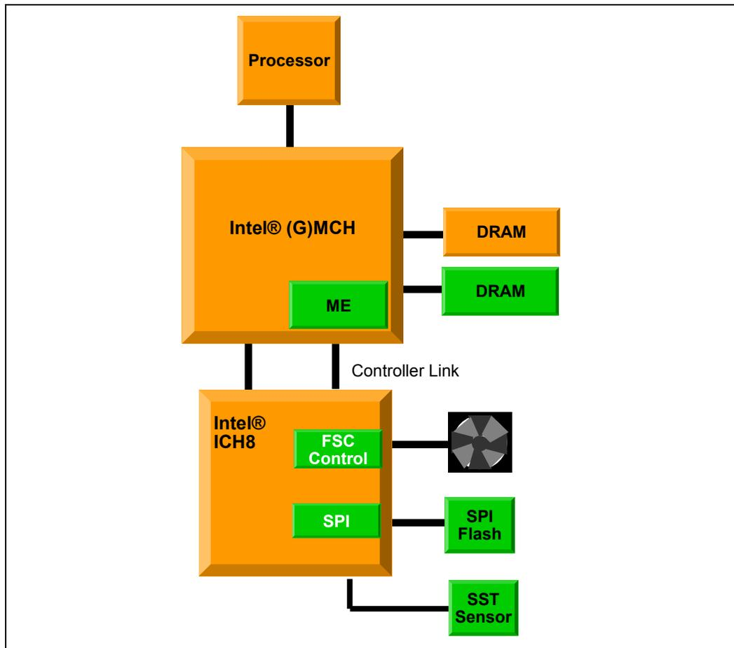
**Note:** Simple Serial Transport (SST) is a single wire bus that is included in the ICH8 to provide additional thermal and voltage sensing capability to the Manageability Engine (ME)
