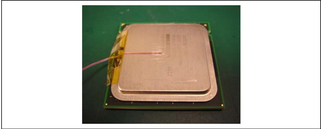
29. Using a blade carefully shave the excess solder above the IHS surface. Only shave in one direction until solder is flush with the groove surface (see Figure 50).
