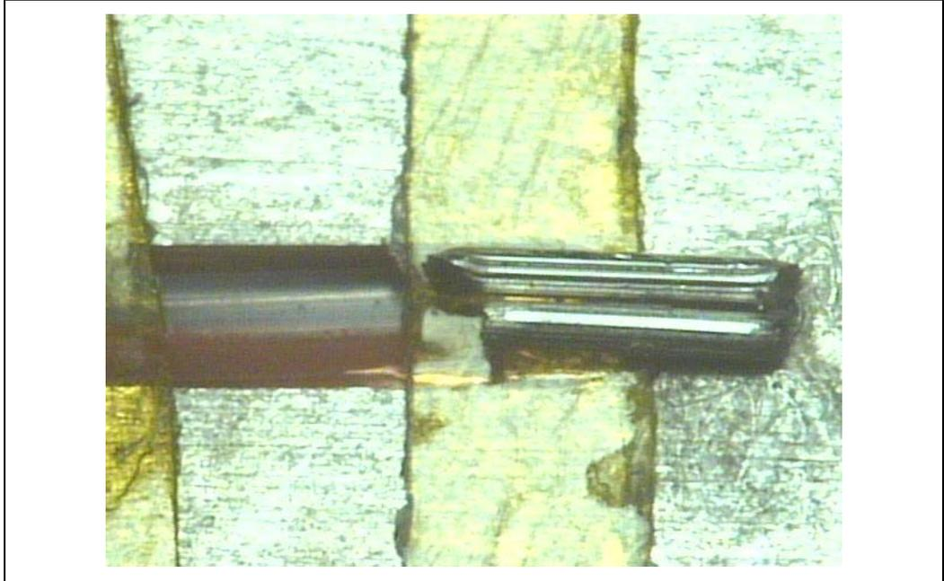
17. Measure the resistance from the thermocouple end wires again using the DMM (refer to Section D.5.1.step 2) to ensure the bead is still properly contacting the IHS.
