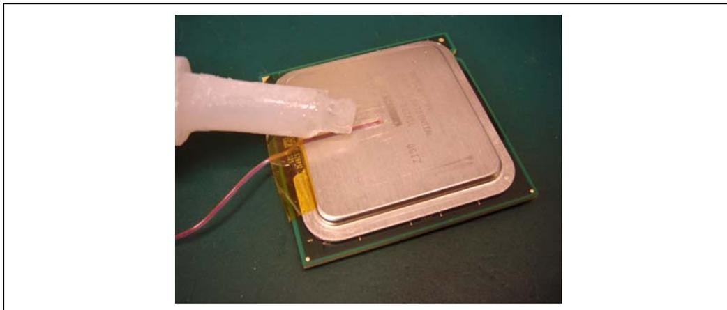
32. To speed up the curing process apply Loctite\* Accelerator on top of the Adhesive and let it set for a couple of minutes (see Figure 52).
