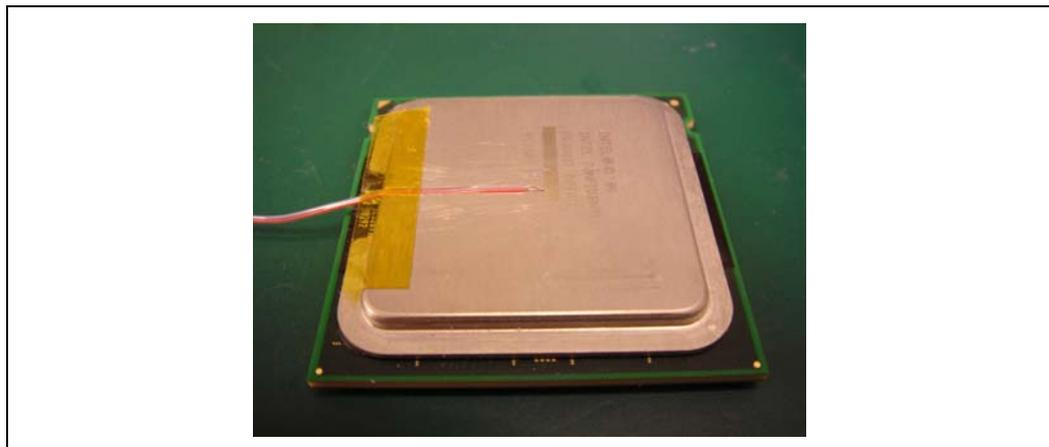
9. Lift the wire at the middle of groove with tweezers and bend the front of wire to place the thermocouple in the groove ensuring the tip is in contact with the end and bottom of the groove in the IHS (see Figure 37-A and B).
