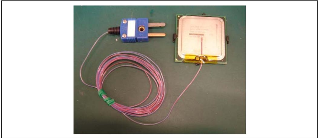
39. Place the device in a tray or bag until it's ready to be used for thermal testing use.
