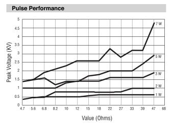
1.2/50  $\mu$ s Peak Voltage Limit (10 pulses at 10 sec. intervals,  $\Delta R < 5$  %)
