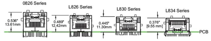
MagJack's Mechanical Evolution Continues to Provide More Efficient Space Utilization with Ultra-Low Profile Packages and Mid-Plane Mount Versions.
