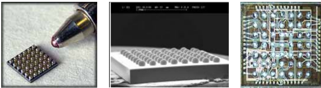
Figure 1. WLCSP Packages Available from Freescale
