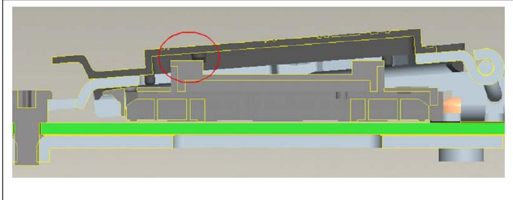
As indicated in [Figure 4-7](#), the pick and place cover cannot remain in place and used in conjunction with the ILM Cover. The ILM Cover is designed to interfere and pop off if the pick and place cover is unintentionally left in place. The ILM cover will also interfere and pop off if the ILM is closed with a processor in place in the socket.
