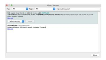
Now you are ready to test! Open up the IDE and load File $\rightarrow$ Examples $\rightarrow$ RGBmatrixPanel $\rightarrow$ testcolors\_16x32 (for the 16x32 panel) or File $\rightarrow$ Examples $\rightarrow$ RGBmatrixPanel $\rightarrow$ colorwheel\_32x32 (for the 32x32 panel).
