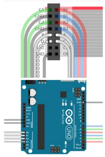
Pins A, B, C and D select which two rows of the display are currently lit. (32x16 matrices don't have a "D" pin — it's connected to ground instead.)
