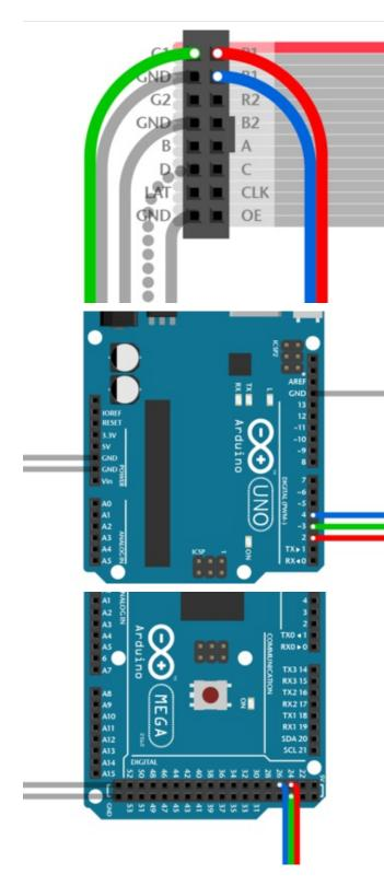
Pins **R1**, **G1** and **B1** (labeled R0, B0 and G0 on some matrices) deliver data to the **top half** of the display.
