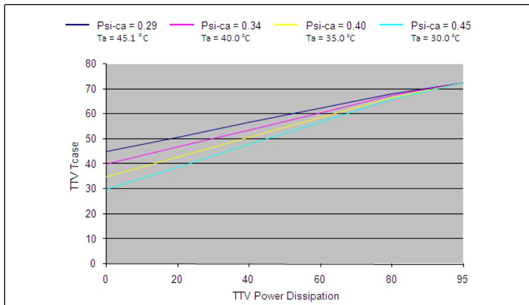
**Note:** If an ambient of greater than 45.1 °C is necessary based on the boundary conditions a thermal solution with a  $\Psi_{CA}$  lower than 0.29 °C/W will be required.
