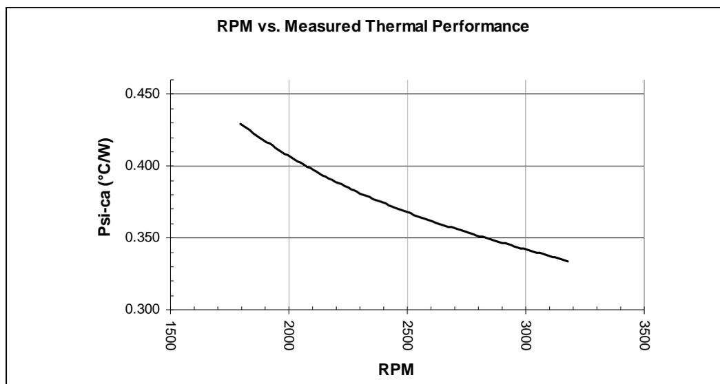
**Note:** This data is taken from the preliminary evaluation of the validation of the RCBF7-1156 (DHA-A) reference processor thermal solution. The  $\Psi_{CA}$  versus RPM data is available in [Table 8-3](#) at the end of this chapter.
