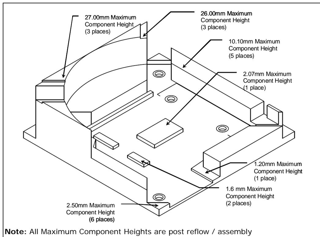
**Note:** The maximum height of the reference thermal solution (in Figure 9-2) above the motherboard is 46.00 mm [1.81 inches], and is compliant with the motherboard primary side height constraints defined in the *ATX Specification* and the *microATX Motherboard Interface Specification* found at <http://www.formfactors.org>.
