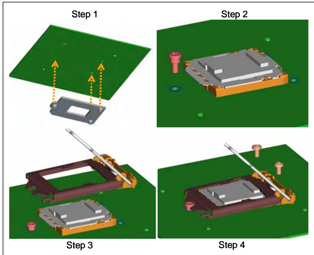
As indicated in [Figure 4-5](#), the shoulder screw, socket protrusion and ILM key features prevent 180 degree rotation of ILM cover assembly with respect to socket. The result is a specific Pin 1 orientation with respect to ILM lever.
