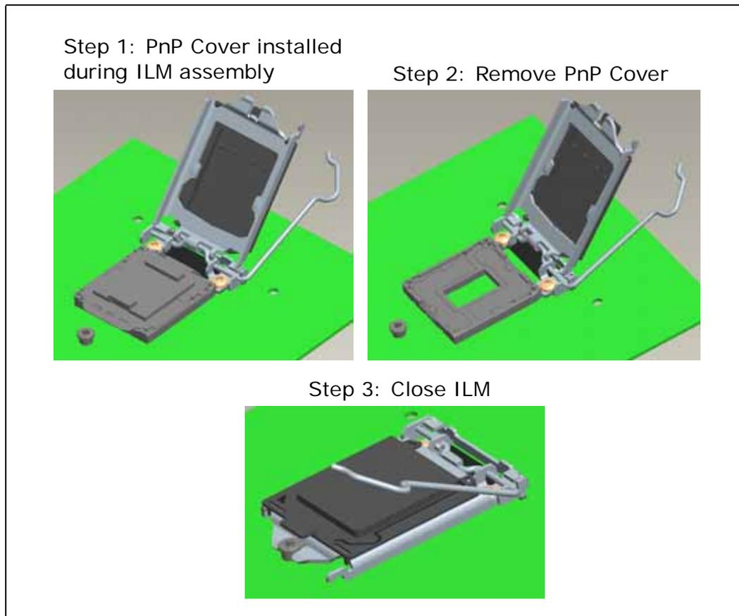
As indicated in [Figure 4-6](#), the pick and place cover should remain installed during ILM assembly to the motherboard. After assembly, the pick and place cover is removed, the ILM Cover installed and the ILM mechanism closed. The ILM Cover is designed to pop off if the pick and place cover is accidentally left in place and the ILM closed with the ILM Cover installed. This is shown in [Figure 4-7](#).
