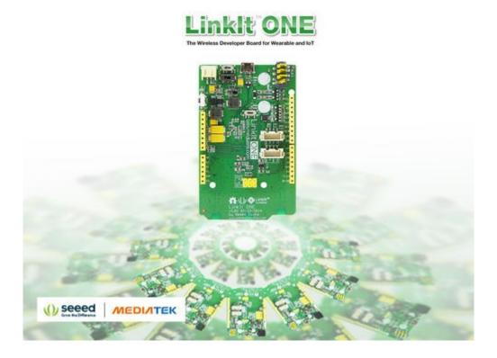
The LinkIt ONE development platform is an open source, high performance board for prototyping Wearables and IoT devices. It is based on the world's leading SoC for Wearables, MediaTek Aster (MT2502) combined with high performance Wi-Fi (MT5931) and GPS (MT3332) chipsets to provide you with access to all the features of MediaTek LinkIt. It also provides similar pin-out features to Arduino boards, making it easy to connect various sensors, peripherals, and Arduino shields.
