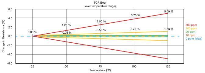
The following equation calculates the maximum change in resistance value for a given TCR.
