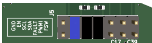
Figure 21. EN pin connection: to MCU or manually to GND
