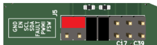
Figure 21. EN pin connection: to MCU or manually to GND
