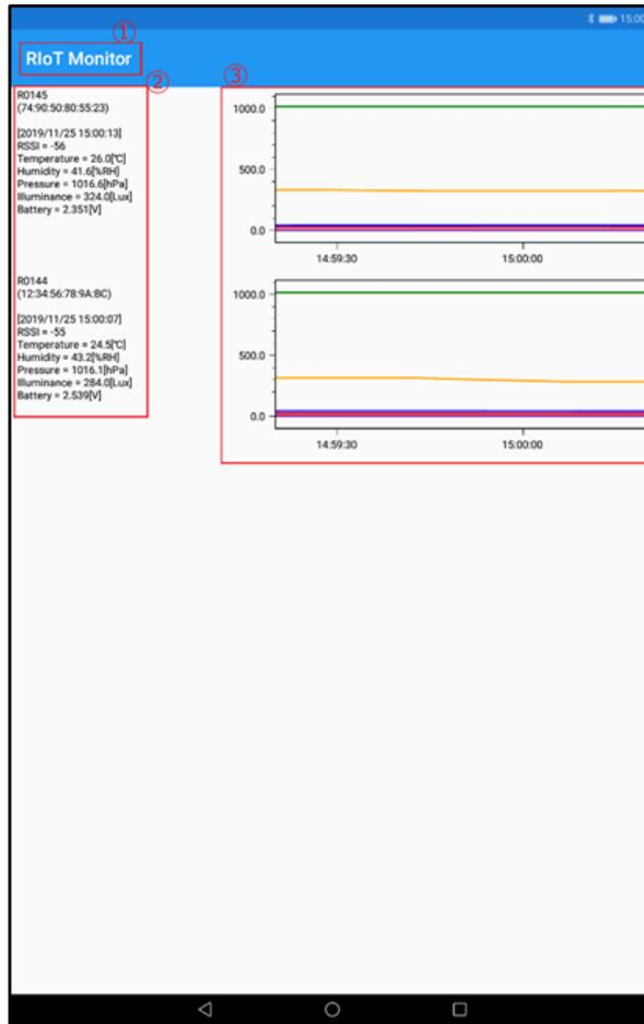
Figure 14 Main Display screen of RIoT\_Monitor
