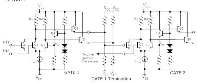
It is important that both outputs are terminated for best performance. If only one output is used, the duty cycle and jitter can be adversely affected.
