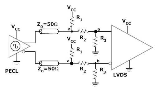
There is not an exact solution for 3.3V. Here are optimum values to use: for 2.5V the schematic must change, move R1 from VCC to 'b' and move R3 from 'a' to ground.
