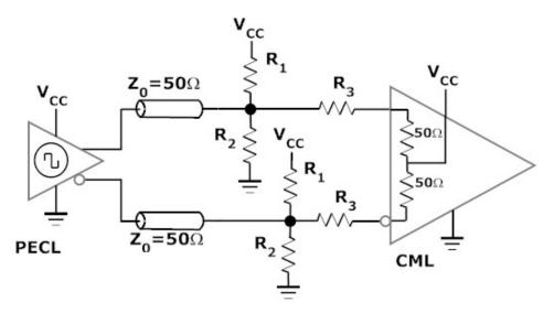
The  $V_{\text{CM}}$  of the CML input and the signal swing on the CML input will need to use the minimum levels allowed. The CML input is reduced to about 0.125V PP which is still within the CML input minimum level specification. Therefore R3 is 275 ohms.
