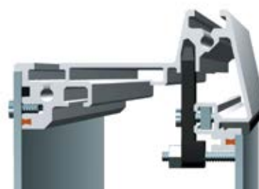
Front panel installation with stud bolts
