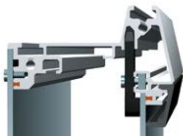
Front panel installation from rear
