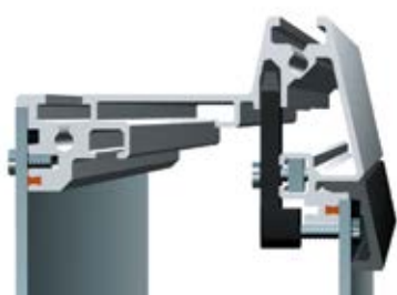
Front panel installation screwed from front
