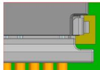
When the terminal contacts are not exposed, it indicates the crimp housing is completely mated to the receptacle.
