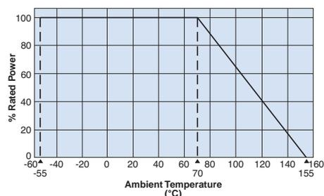
For resistors operated at an ambient temperature of 70°C or above, the power rating shall be derated in accordance with the above derating curve.
