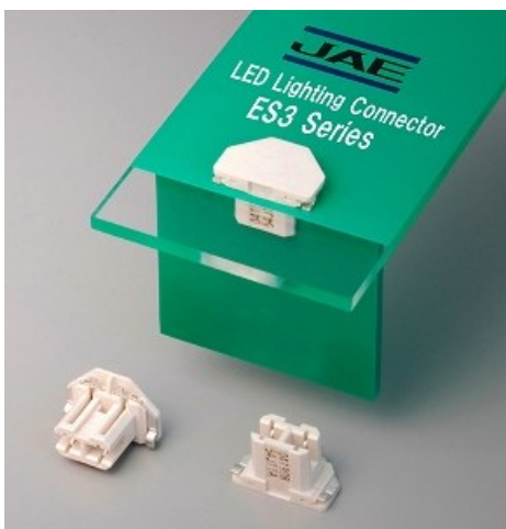
JAE's ES3 Series card edge LED lighting connector is made with white plastic molding which maximizes light emission by reflecting light rather than absorbing it.
