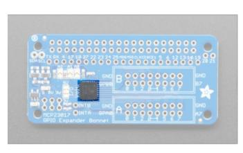
The **MCP23017 GPIO expander chip** converts Python code into pin instructions.
