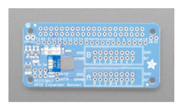
This Bonnet defaults to using 5V. There is a jumper to swap between 3V and 5V. If you want to change it to 3V, you can cut the trace between the top two pads, and solder the bottom two pads.
