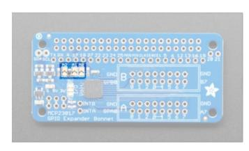
By soldering closed the **address select jumpers**, you can change the address from **0x20 to 0x27**. This allows up to 8 bonnets for 128 total GPIO.
