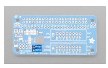
The MCP23017 has interrupt capabilities. There are two IRQ pins (INTA and INTB) you can solder a wire to, if you want to have a quick way of telling if any of the GPIO's changed.
