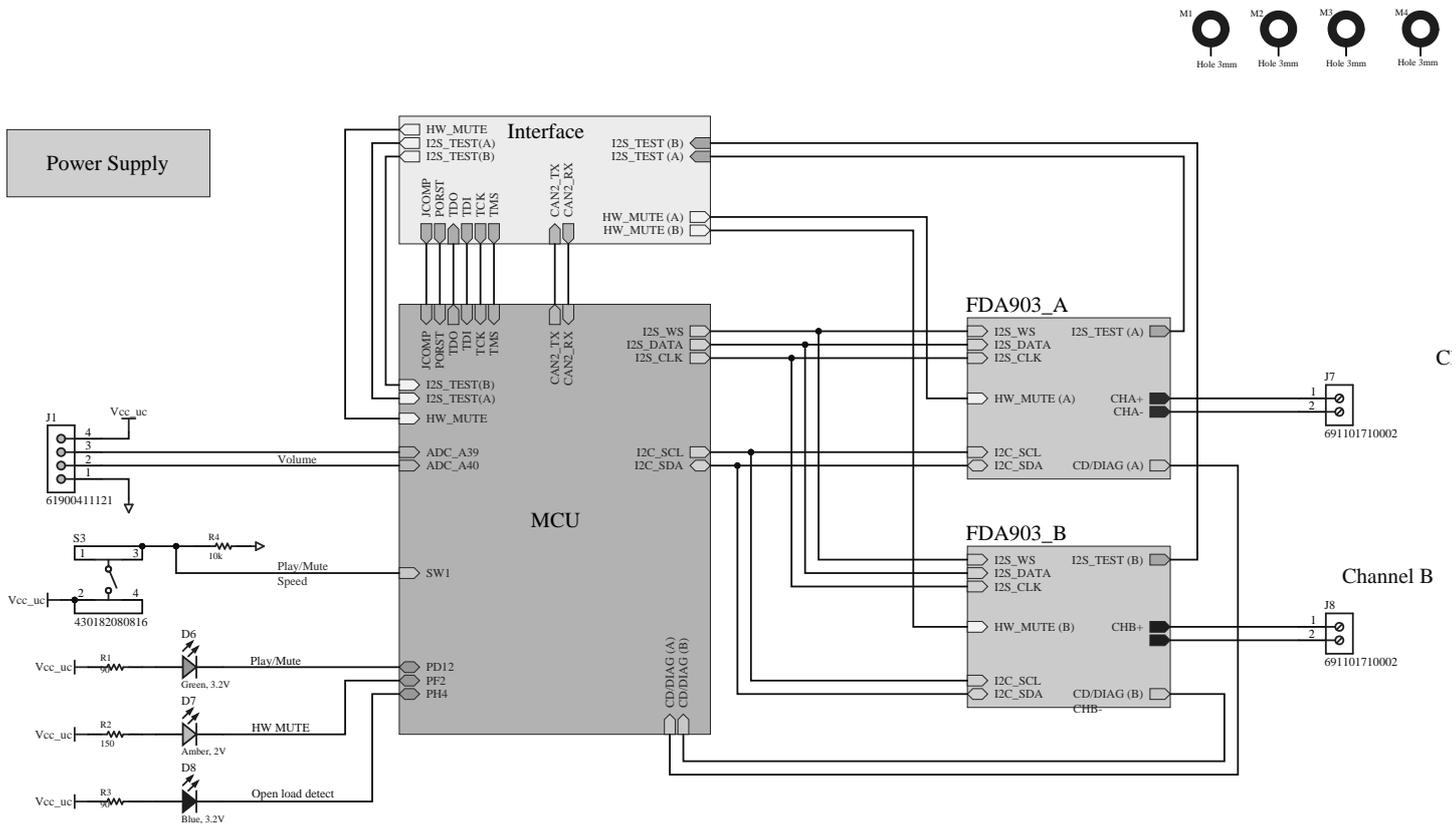
Figure 2: AEK-AUD-C1D9031 circuit schematic (2 of 6)
