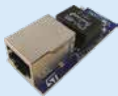
STEVAL-POE001V1 Power Over Ethernet (PoE) - IEEE 802.3bt compliant interface
