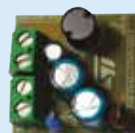
STEVAL-ISA178V1 5 V / 0.2 A buck converter
