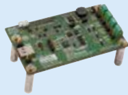
STEVAL-ISC005V1 STUSB4500 USB Power Delivery controller evaluation board
