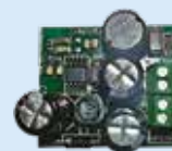
STEVAL-ISA115V1 12 V, 150 mA buck converter
