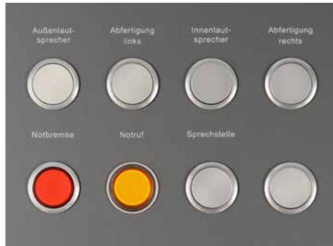
Modern flush-mount pushbutton controls within a train cockpit.
