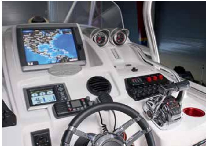
An HMI System provides alarm, status, and performance information for a variety of vessel systems.
