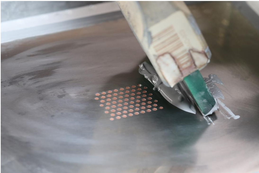
Figure 12 Suggested Squeegee Application Angle
