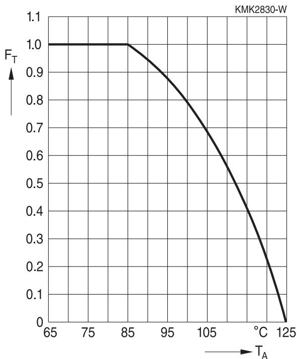
Maximum  $I_{RMS}$  current as function of the ambient temperature:  $I_{RMS}(T_{\text{amb}}) = \text{Factor} \times I_{RMS}(85^\circ\text{C})$
