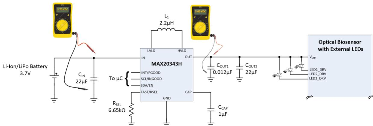
Figure 32. Analog 5VDC MAX20343H SMPS Circuit for Wearable Medical Applications
