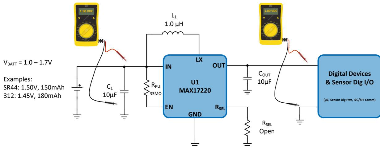
Figure 22. Digital 1.8VDC MAX17220 SMPS Circuit for Wearable Medical/Healthcare Applications
