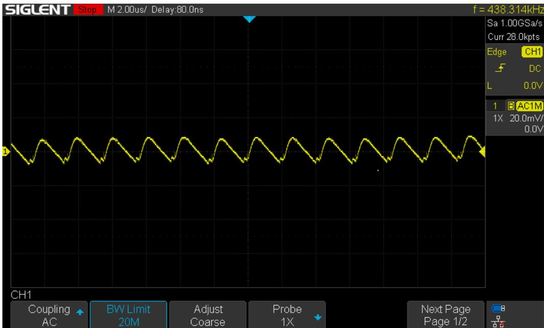
Figure 31: MAX17220 Output Ripple Waveform with 45mA Load Current
