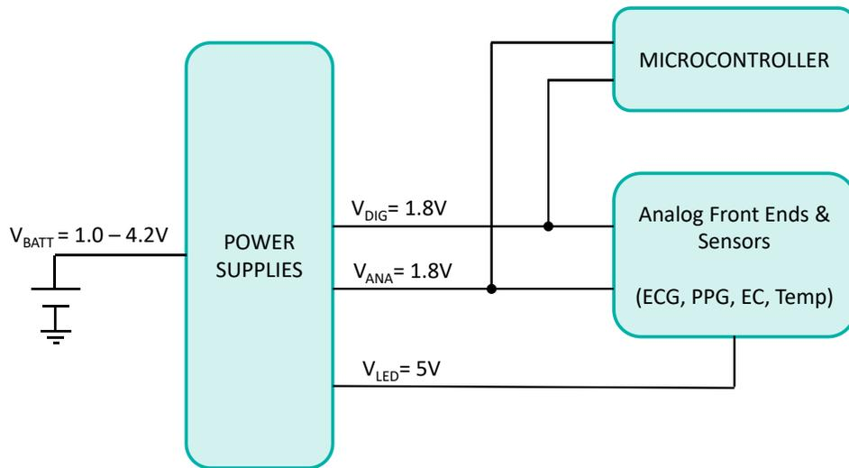
Figure 1. Typical Power Supply Configuration
