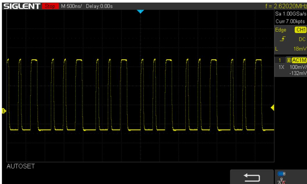
Figure 56. Typical MAX77642 LXA Waveform (SSB0 & SSB1  $I_{OUT} = 1.2\text{mA}$ ; SSB2  $I_{OUT} = 126.1\text{mA}$ )
