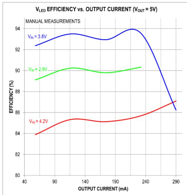
Figure 52. Efficiency of the Analog 5V MAX77642 SMPS Circuit
