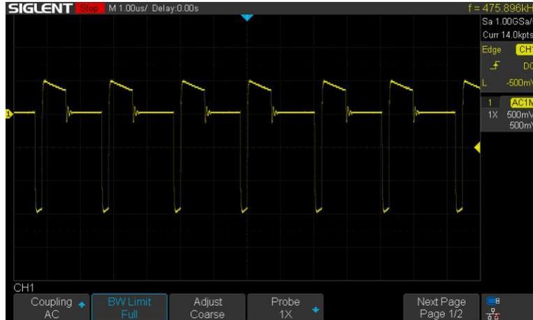
Figure 29: Typical MAX17220  $V_{LX}$  Waveform with 45mA Load.
