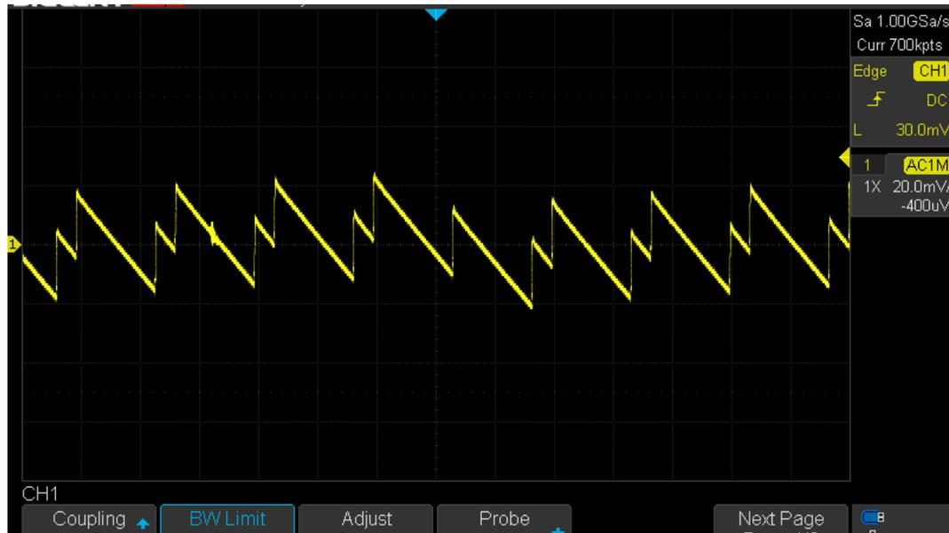
Figure 25. Typical Output Ripple Characteristic ( $V_{IN} = 1.5VDC$ ,  $I_S = 2mA$ )
