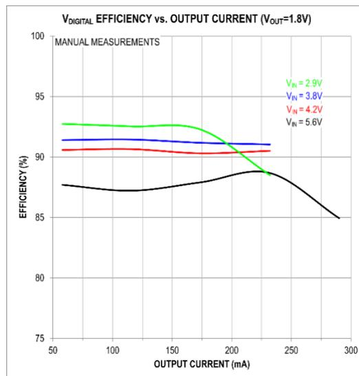
Figure 44. Efficiency of the Digital 1.8V MAX77642 SMPS Circuit
