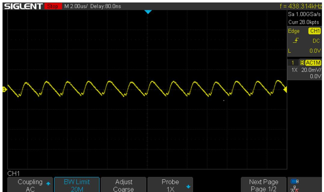
Figure 26. Typical Output Ripple Voltage ( $V_{IN} = 1.5VDC$ ,  $I_S = 45mA$ )
