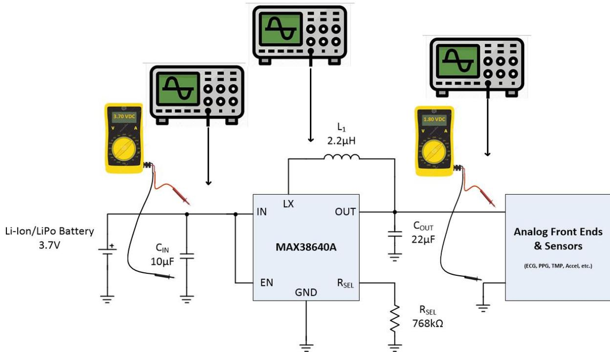
Figure 7. Troubleshooting the MAX38640A SMPS Circuit
