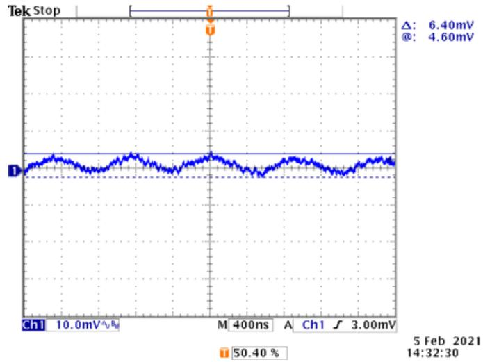
Figure 5. Typical Output Ripple Characteristic ( $V_{IN} = 4.2VDC$ ,  $I_S = 100mA$ )
