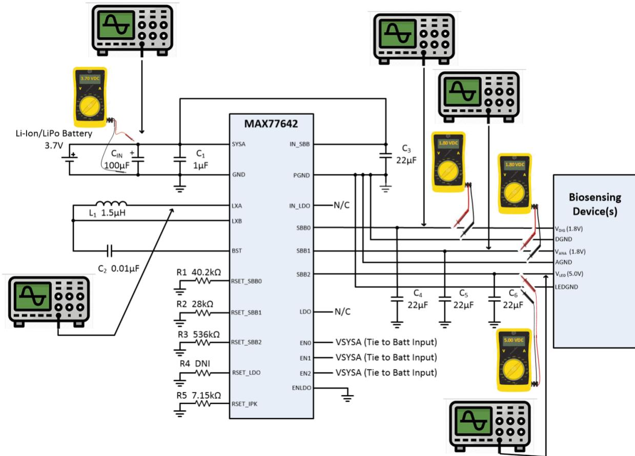
Figure 55. Troubleshooting the MAX77642 SMPS Circuit
