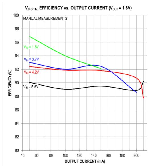
Figure 14. Efficiency of the Digital 1.8V MAX38640A SMPS Circuit
