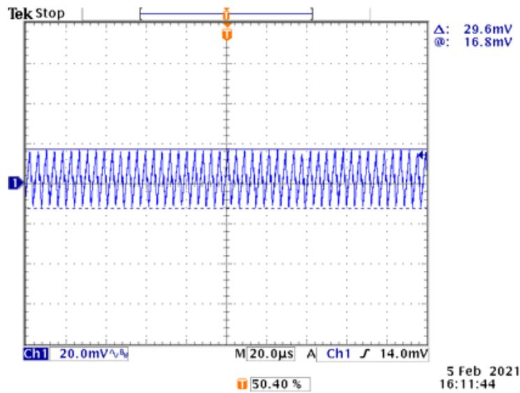
Figure 46. Typical Output Ripple Voltage ( $V_{IN} = 4.2\text{VDC}$ ,  $I_S = 100\text{mA}$ )
