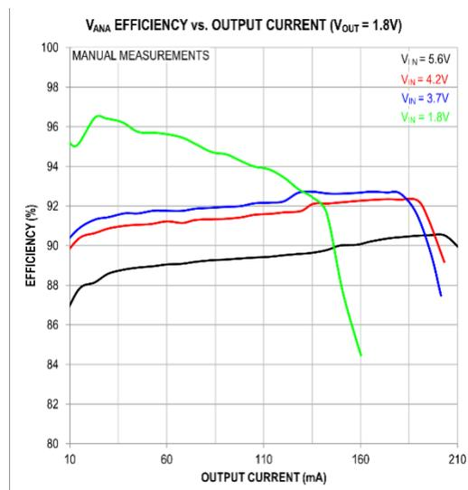
Figure 4. Efficiency of Analog 1.8V MAX38640A SMPS Circuit
