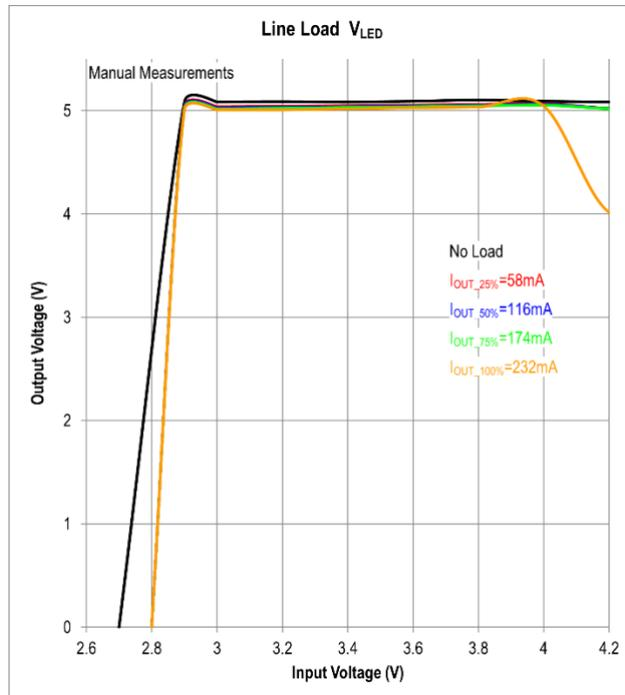
Figure 51. Line Load of the Analog 5V MAX77642 SMPS Circuit
