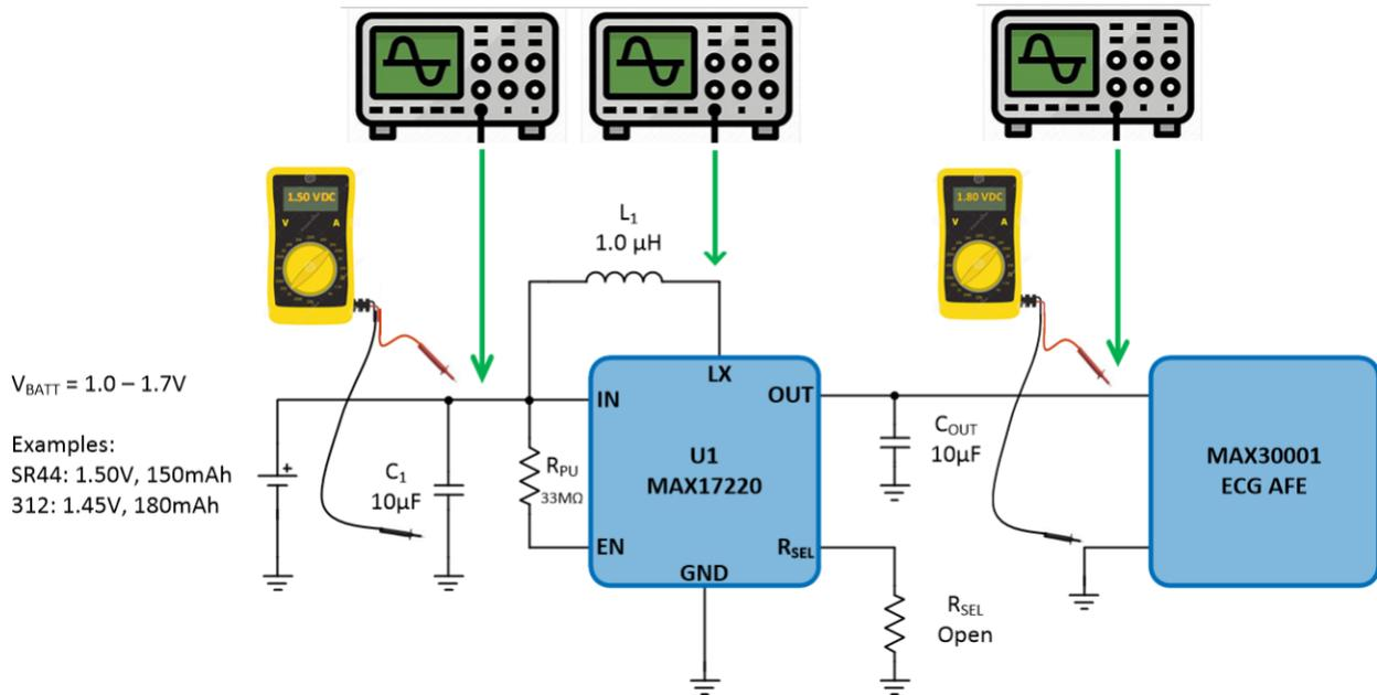
Figure 27: Troubleshooting the MAX17220 SMPS Circuit
