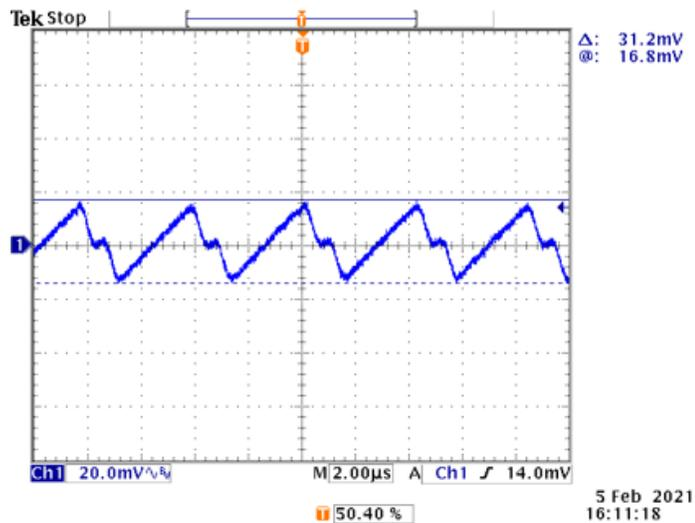
Figure 57. MAX77642 SSB0 (Dig 1.8V) Ripple Waveform ( $V_{IN} = 4.2V$ ,  $I_{OUT} = 100mA$ )
