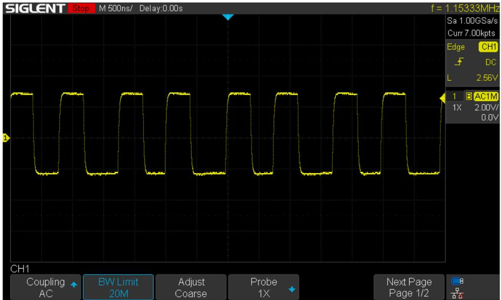
Figure 39. Typical MAX20343H HVLX Waveform with 125mA Load
