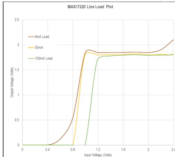
Figure 23. Line Load for the Digital MAX17220 SMPS Circuit
