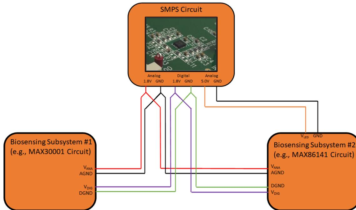
Figure 60. Power Supply "Star" Routing Topology
