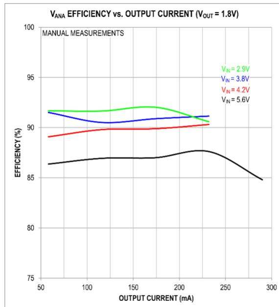
Figure 48. Efficiency of the Analog 1.8V MAX77642 SMPS Circuit
