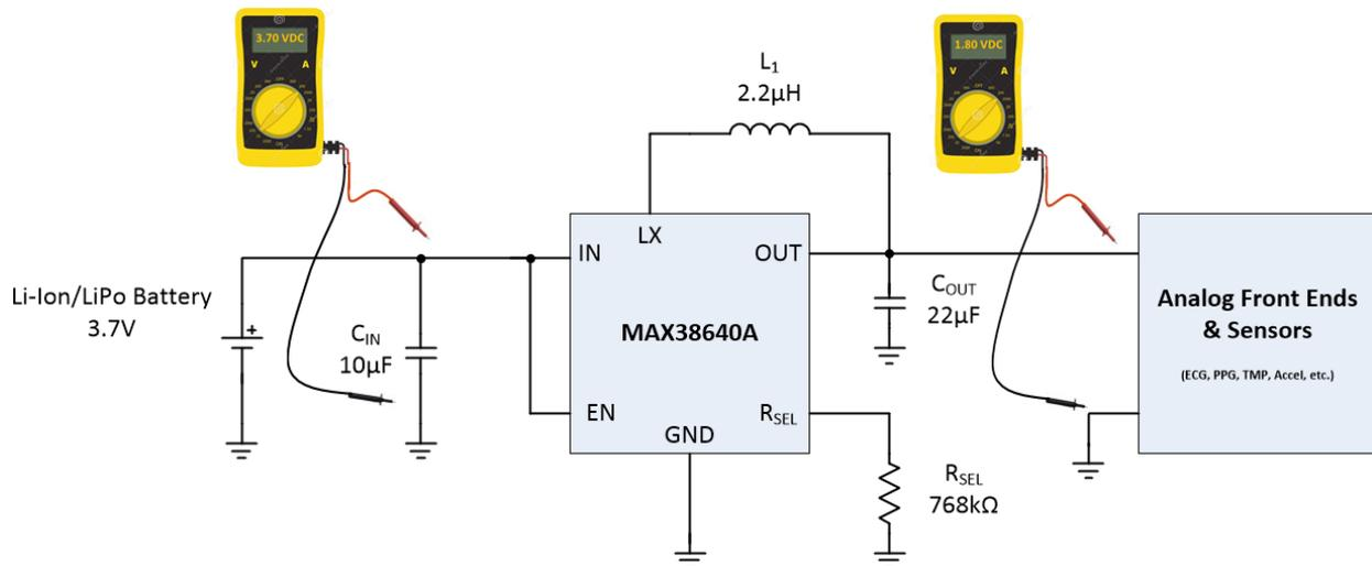
Figure 2. Analog 1.8VDC MAX38640A SMPS Circuit for Wearable/Healthcare Applications
