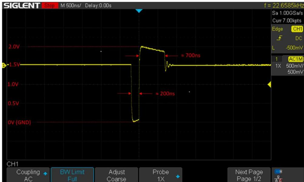
Figure 28: Typical MAX17220  $V_{LX}$  Waveform with 2mA Load
