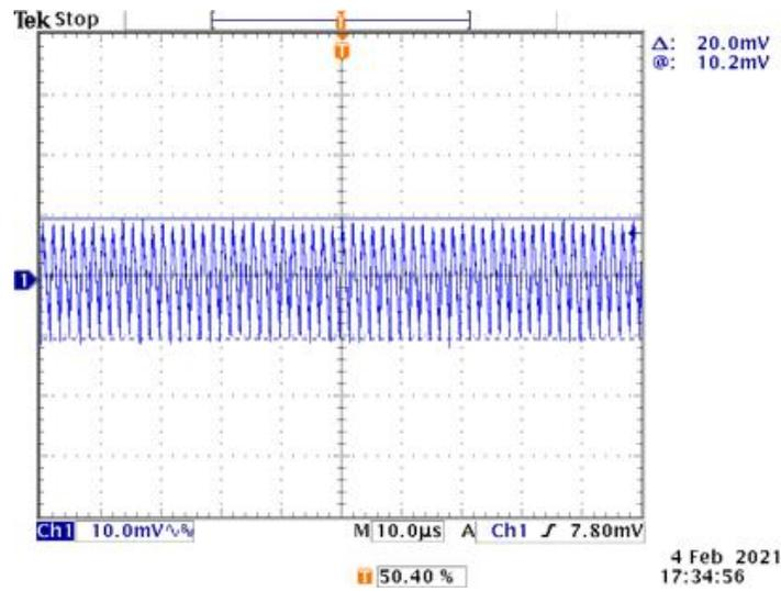
Figure 36. Typical Output Ripple Voltage ( $V_{IN} = 4.2\text{VDC}$ ,  $I_S = 100\text{mA}$ )
