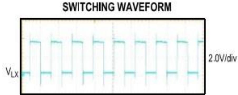
Figure 19. Typical MAX38640A VLX Waveform
