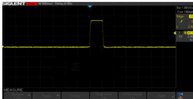
Figure 38. Typical MAX20343H HVLX Waveform with Light Load (10mA)
