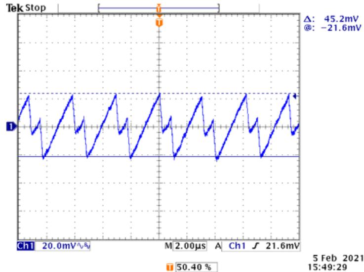
Figure 59. MAX77642 SSB2 (5.0V) Ripple Waveform ( $V_{IN} = 4.2V$ ,  $I_{OUT} = 100mA$ )
