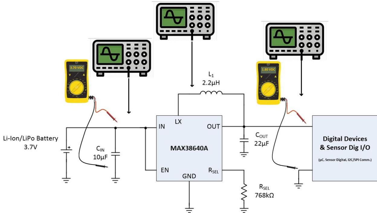
Figure 17. Troubleshooting the MAX38640A SMPS Circuit
