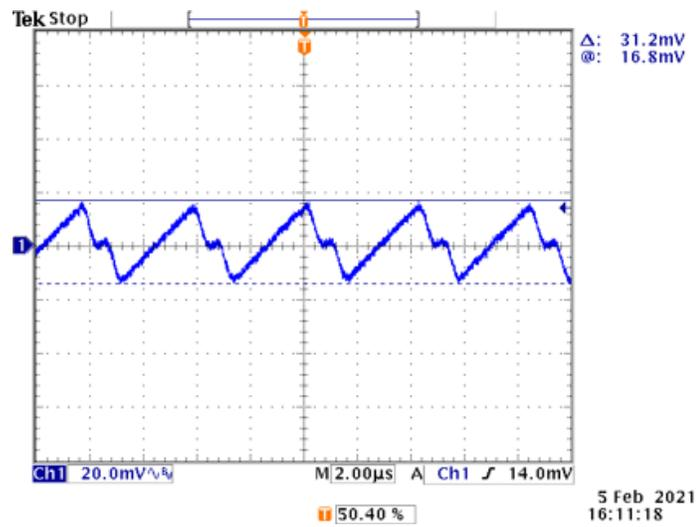
Figure 45. Typical Output Ripple Characteristic ( $V_{IN} = 4.2\text{VDC}$ ,  $I_S = 100\text{mA}$ )
