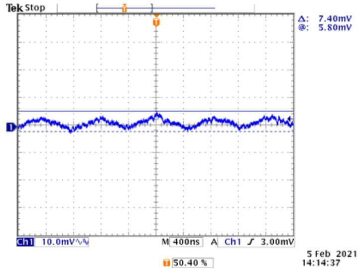
Figure 15. Typical Output Ripple Characteristic ( $V_{IN} = 4.2VDC$ ,  $I_S = 100mA$ )
