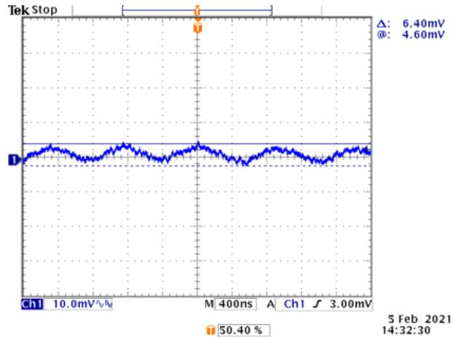
Figure 11. MAX38640A Output Ripple Waveform
