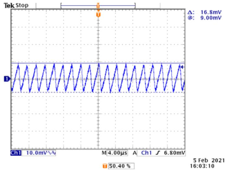
Figure 50. Typical Output Ripple Voltage ( $V_{IN} = 4.2\text{VDC}$ ,  $I_S = 100\text{mA}$ )
