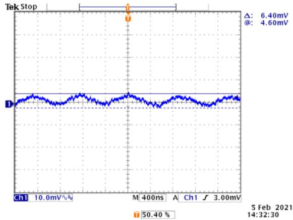
Figure 21. MAX38640A Output Ripple Waveform
