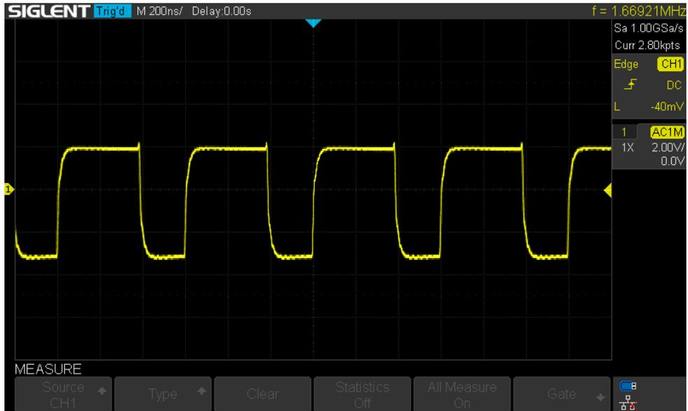
Figure 40. Typical MAX20343H HVLX Waveform with 246mA Load
