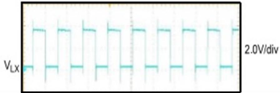
Figure 9. Typical MAX38640A VLX Waveform
