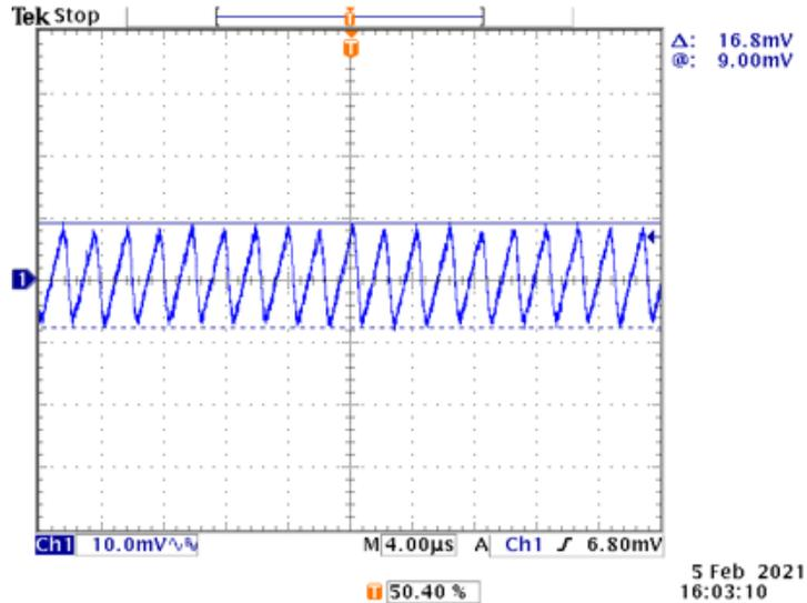
Figure 58. MAX77642 SSB1 (Analog 1.8V) Ripple Waveform ( $V_{IN} = 4.2V$ ,  $I_{OUT} = 100mA$ )
