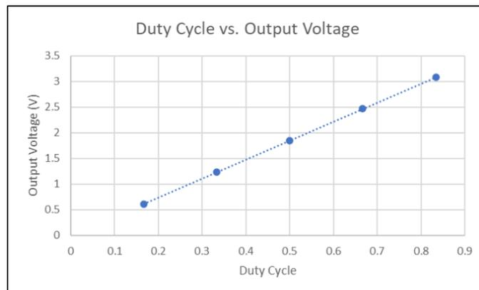
Figure 10. MAX38640A Duty Cycle Versus Output Voltage
