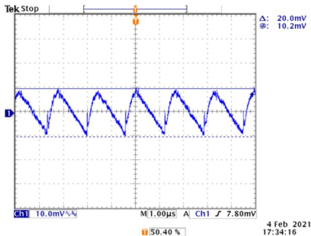
Figure 41. MAX20343H (5V) Output Ripple Waveform
