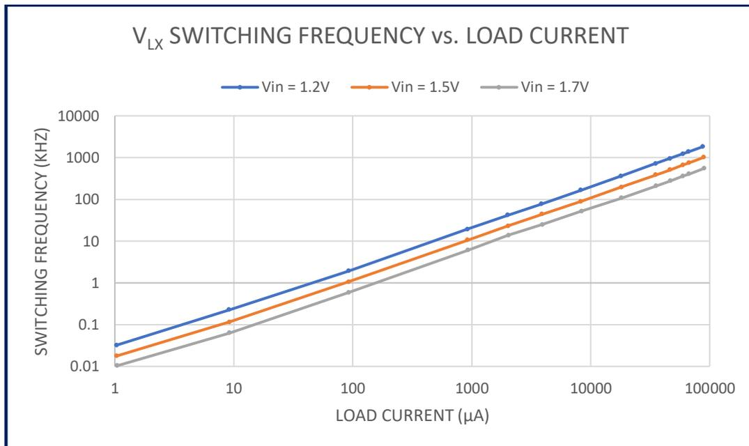
Figure 30: MAX17220  $V_{LX}$  Frequency vs. Load Current
