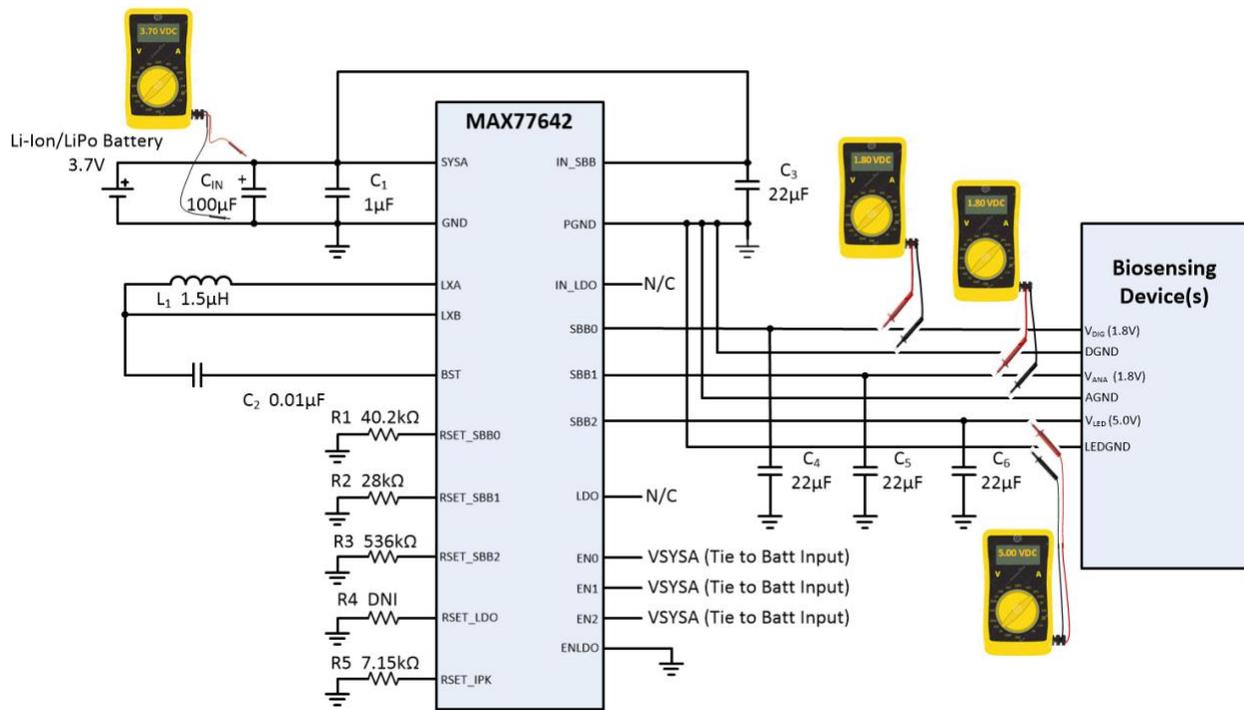
Figure 42. Analog 1.8V/Digital 1.8V/Analog 5.0V MAX77642 SMPS Circuit for Wearable Medical Applications
