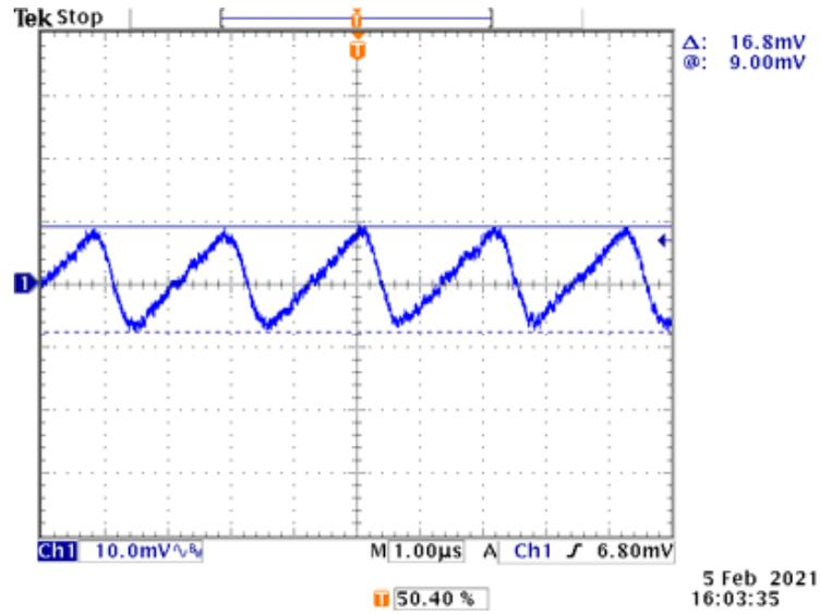
Figure 49. Typical Output Ripple Characteristic ( $V_{IN} = 4.2\text{VDC}$ ,  $I_S = 100\text{mA}$ )
