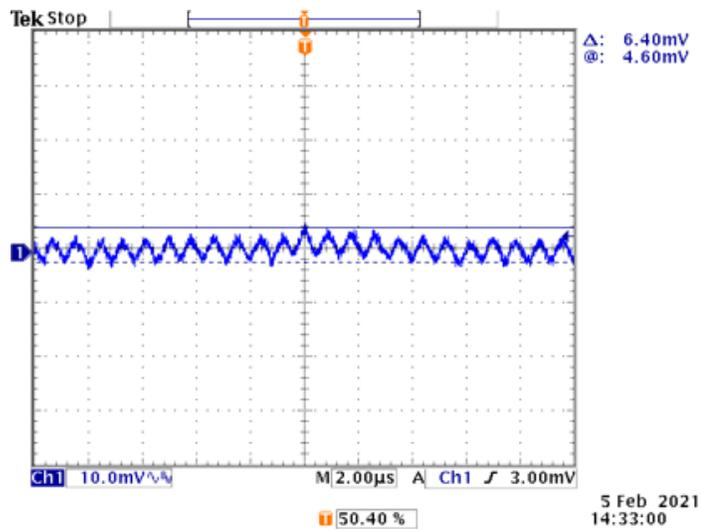
Figure 6. Typical Output Ripple Voltage ( $V_{IN} = 4.2VDC$ ,  $I_S = 100mA$ )
