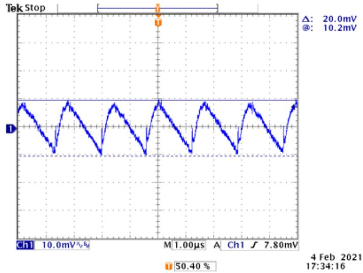
Figure 35. Typical Output Ripple Characteristic ( $V_{IN} = 4.2\text{VDC}$ ,  $I_S = 100\text{mA}$ )
