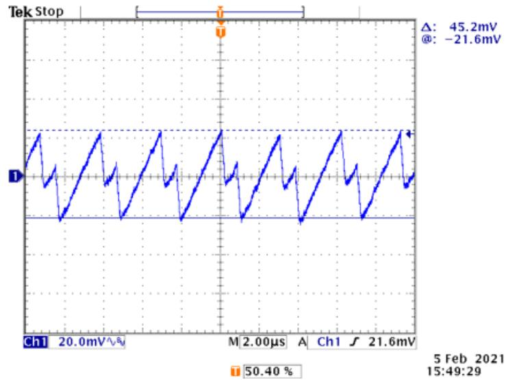
Figure 53. Typical Out Ripple Characteristic ( $V_{IN} = 4.2\text{VDC}$ ,  $I_S = 100\text{mA}$ )
