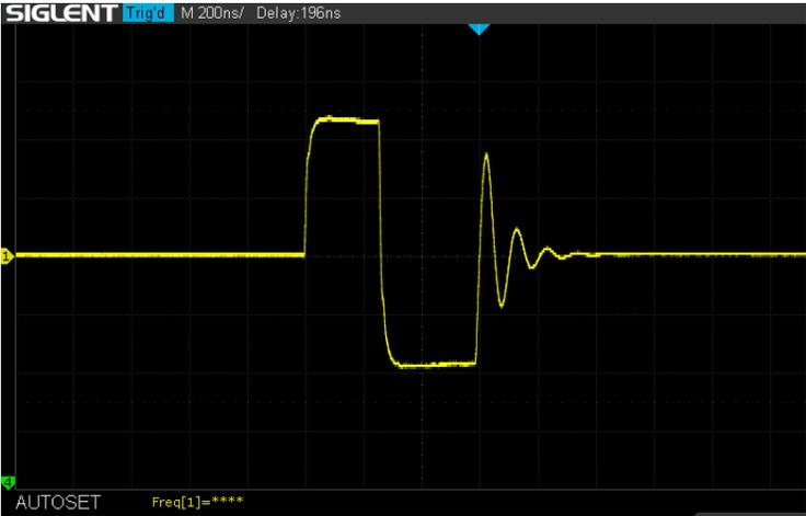
Figure 18. Typical MAX38640A VLX Waveform with Light Load
