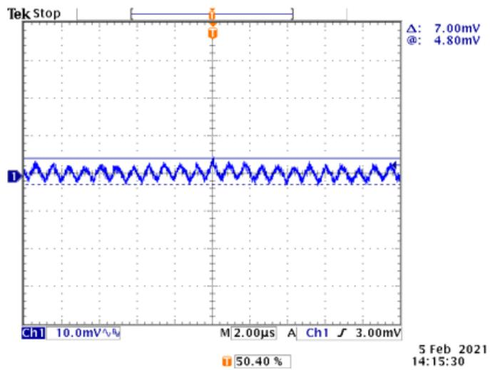
Figure 16: Typical Output Ripple Voltage ( $V_{IN} = 4.2VDC$ ,  $I_S = 100mA$ )
