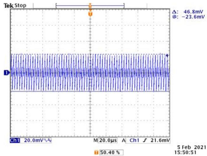
Figure 54. Typical Output Ripple Voltage ( $V_{IN} = 4.2\text{V}$ ,  $I_S = 100\text{mA}$ )
