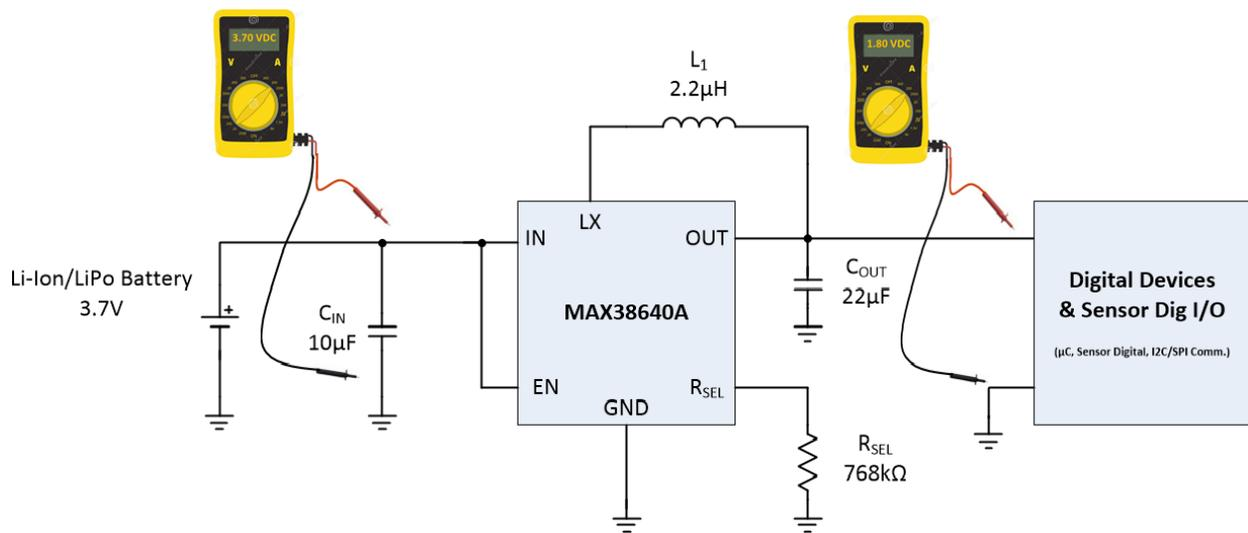
Figure 12. Digital 1.8VDC MAX38640A SMPS Circuit for Wearable Medical/Healthcare Applications
