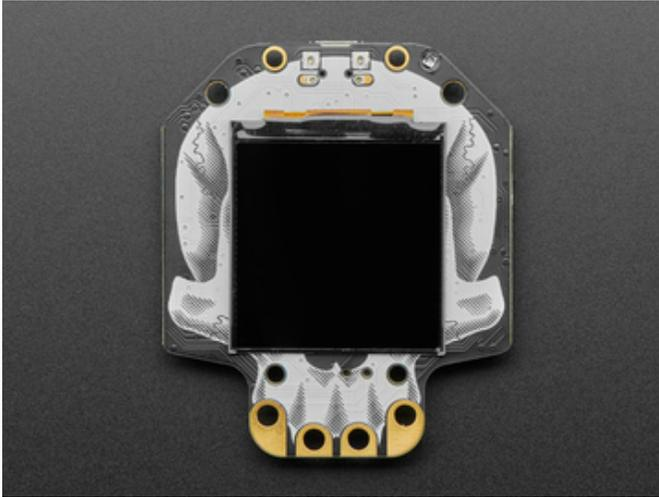
On the front is a **1.54"** sized **240x240** full color IPS TFT. Compared to the HalloWing M0's 1.44" 128x128, this has 4x as many pixels and is IPS for great color and brightness.
