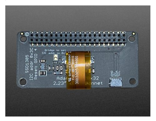
Comes completely pre-assembled and tested so you don't need to do anything but plug it in and install our Python code! Works with any Raspberry Pi computer that has a 2x20 connector, such as the Pi B+, Pi 2, Pi 3, Pi 4, and Pi Zero (and any others that have a 2x20 connector!)
