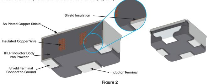
The Vishay IHLE inductors eliminate the need to cover the whole circuit in an expensive Faraday cage. The integrated shield stops the radiation of the E-field and virtually eliminates the B-field.
