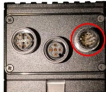
\*Note if you are using an external flying lead – m12 cable please verify the Pinouts with the wiring diagram
