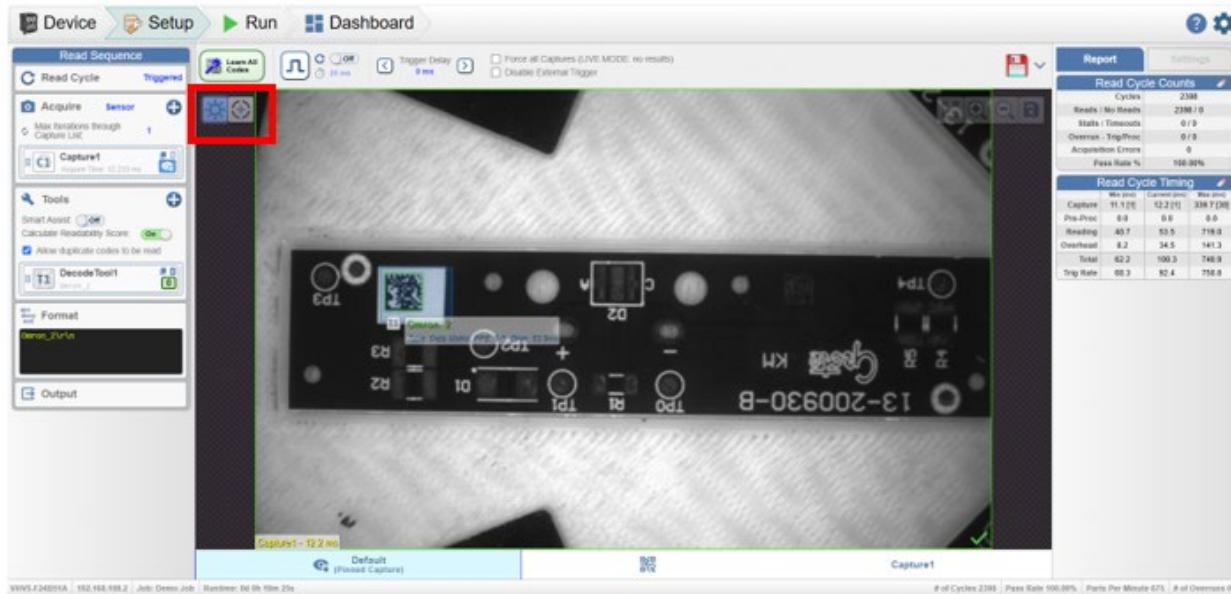
The reader will cycle through multiple Image captures to select the proper exposure time.
