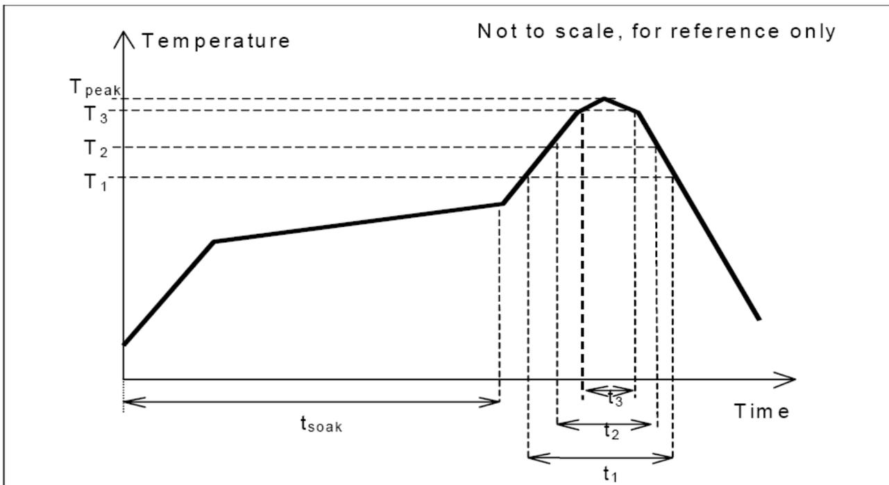
This profile is the minimum requirement for evaluating soldering heat resistance of components. Heat transfer method used for reflow soldering is hot air convection. The actual air temperatures used to achieve the specified profile is higher and largely dependent on the reflow equipment.
