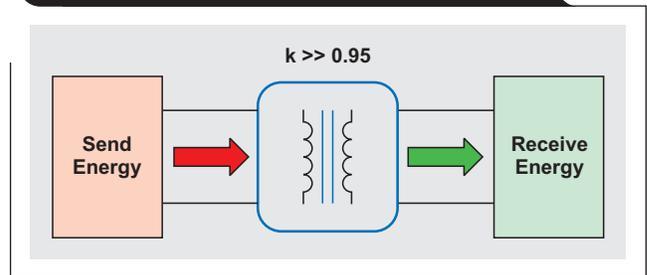
**Figure 2. Ideal model of a traditional transformer**
