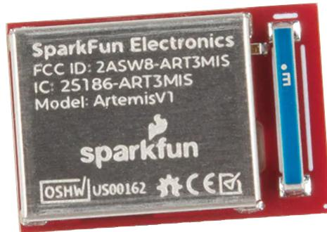
The WRL-15484 Artemis module is fully certified by FCC/IC/CE and has 48 all interrupt capable GPIOs and a secure smart card interface. This module can be easily implemented into any design using low-cost 2-layer PCBs and 8mil trace/space.
