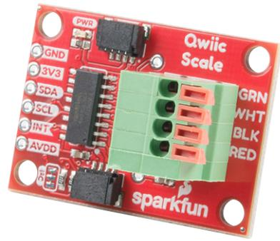
The Qwiic scale board provides a four spring terminal to connect the load cell with no soldering required. This board also breaks out an interrupt pin and AVDD to the edge of the board in addition to the I<sup>2</sup>C pins.
