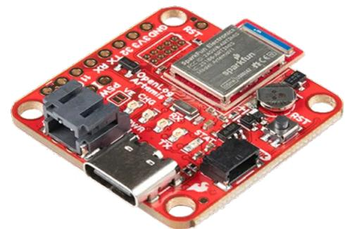
The OpenLog Artemis is highly configurable over an easy-to-use serial interface. Simply plug in a USB-C cable and open a terminal at 115200bps. The logging output is automatically streamed to both the terminal and the microSD. This board automatically scans, detects, configures, and logs various Qwiic sensors plugged into the board without the need for soldering and programming.
