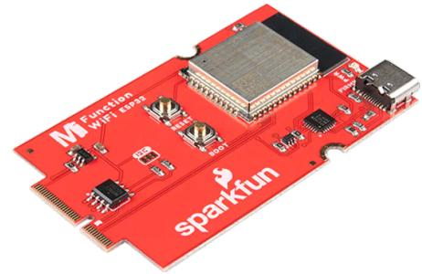
The MicroMod WiFi function board does not require soldering to connect it to any system. The key can be matched to the processor and function board's beveled edge connector to the respective key on the M.2 connector. The ESP32 WROOM module can then be controlled using AT commands via the serial UART port. The USB-C™ connector and CP2102 USB-to-serial converter can be used to add AT commands, flash custom firmware on the ESP32, or reprogram the ESP32.
